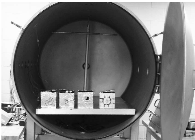
Figure 15 — Balloonsat payloads were placed in a vacuum chamber from which the air was evacuated to simulate a flight to 100,000 feet.
