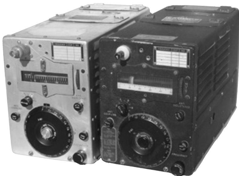
Figure 10 — A pair of 7 to 9.1 MHz ARC-5 transmitters from WWII. On the left is the US Army Air Forces version (BC-459), and a Navy equivalent (T-22, ARC-5) is shown on the right. These were available for about $5 in “new in box” condition after WWII.
