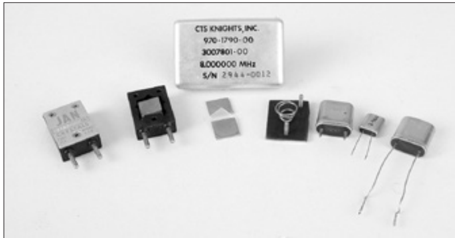
Figure 11 — Sample of typical frequency control crystals for amateur use. The units on the right are modern sealed types. On the far left is a WWII era crystal with a disassembled type FT-243 holder in the center.
