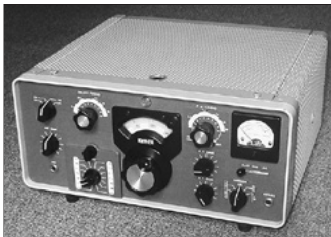
Figure 26 — An early SSB transceiver, the 1957 vintage Collins KWM-2(A). [Photo courtesy of the Collins Collectors Association]
