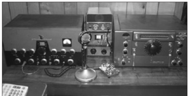
Figure 18 — A typical 1950s amateur AM and CW station used a separate transmitter and receiver. Shown here is W1ZR's 1950s-era station with an E. F. Johnson Viking II transmitter (100 W) with separate VFO on the left and a National HRO-60 receiver on the right.
