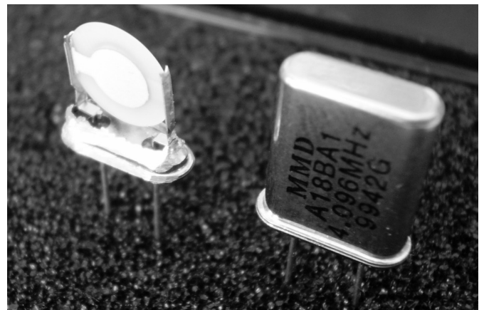
Figure 1 — The internal structure of a quartz crystal unit is shown on the left. The complete package in the metal HC-49U case is shown on the right.
