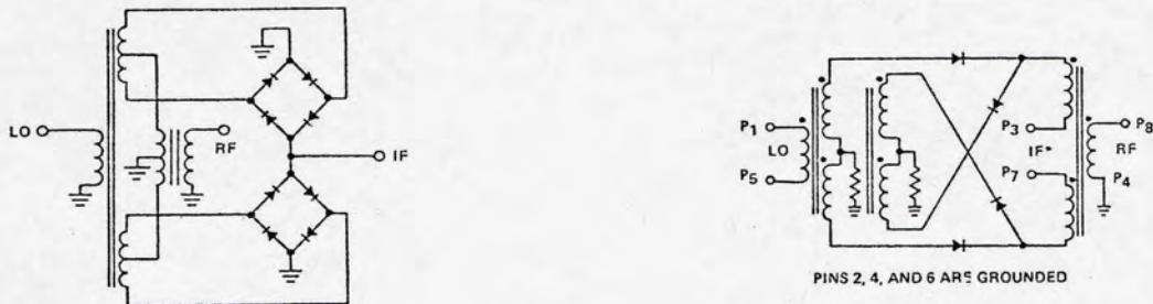
Figure 3a and b - High level double balanced mixer
