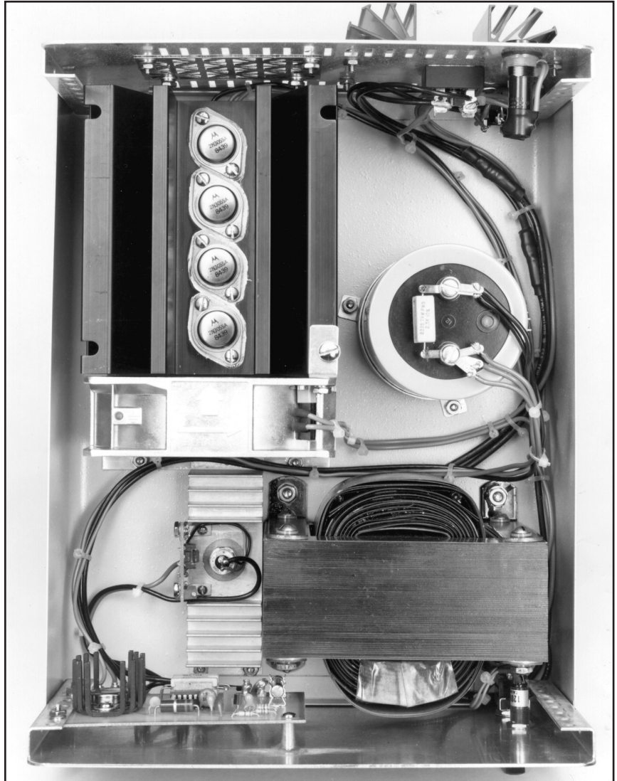
Fig 17.47 — Interior of the 28-V, high-current power supply. The cooling fan is necessary only if the pass transistors and heat sink are mounted inside the cabinet. See text.
