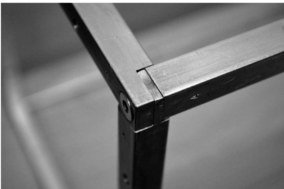
Figure 7 — The rectangular frame is constructed from \frac{1}{2} inch square aluminum stock. A single 10-32 flathead screw secures the three interlocking pieces that form each corner.
