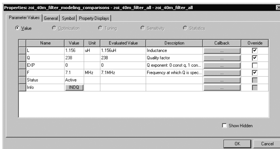
Fig 6.25 — Simulating the 7-MHz filter in Ansoft Designer SV 2 , lets us use inductors that realistically model Q . Doing so then requires us to model the filter's input and output links with ideal transformers characterized in terms of turns ratio. The resonators in the real-world circuit are 17-turn toroidal coils with 2-turn links. The test generator and terminations necessary for SPICE analysis are absent for the reasons described in the text.
