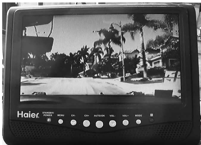
Fig 18 — Mobile ATV as shown here with a portable TV works fine using D-CATV 64-QAM, but it exhibits occasional freeze or tile effect from drop outs and multipath.
