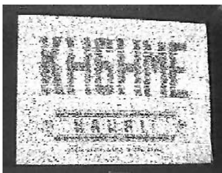
Fig 2 — The one-way ATV DX record is held by KC6CCC in San Clemente, California, for reception of 434-MHz video from KH6HME in Hawaii during a tropo opening in 1994. The distance is 2518 miles. See www.hamtv.com/atvdxrecord.html .
