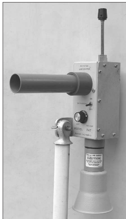
Fig 27.11 — The Radar Engineers Model 247 Hotstick Line Sniffer is an RF and ultrasonic locator. It is used by utility workers to pinpoint the exact piece of hardware causing a noise problem. Mounted on a hotstick, the sniffer is used from the pole or from a bucket.
