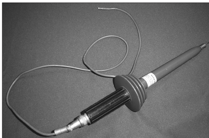
Fig 26.3 — A probe used for measuring high-voltage with a standard multi-meter.
