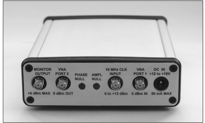
Fig 25.90 — The adapter is built in a standard Hammond extruded aluminum cabinet. Front and rear panels are pictured.
