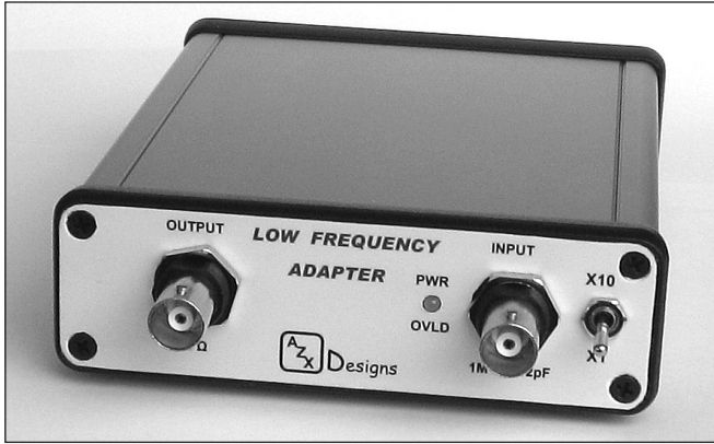
Fig 25.90 — The adapter is built in a standard Hammond extruded aluminum cabinet. Front and rear panels are pictured.
