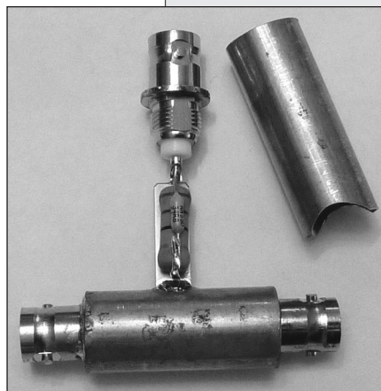
Fig 25.78 — RF sampler using tube construction.
