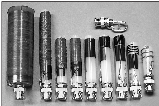
Fig 25.82 — This is how the coils look before covering them with heat-shrink tubing or tape. Small pieces of electrical tape are used to hold the turns in place during construction.
