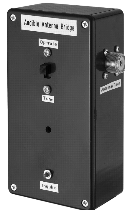
Fig 24.31 — Front view of the audible antenna bridge.
