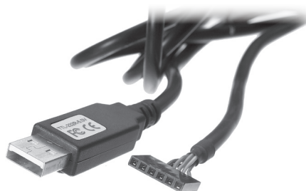
Fig 24.40 — The FTDI TTL-232R cable simplifies construction.
