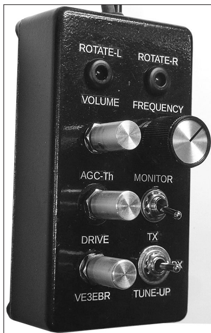
Figure 24.54 — The SDR Knob Box replaces software controls such as click boxes and sliders with physical knobs and switches read by an Arduino micro-controller and then relays the appropriate commands to an SDR transceiver.
