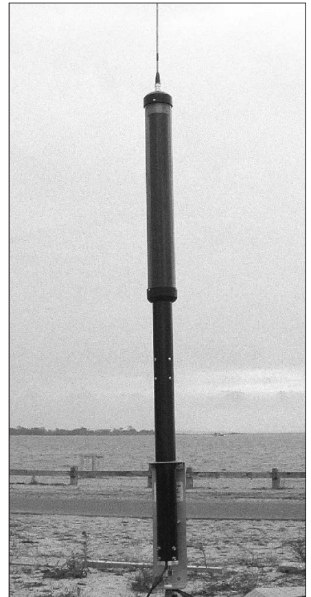
Fig 21.84 — The screwdriver-style remotely-controlled whip antenna. A small motor in the base mast moves a coil past contacts at the top of the metal base section. The top whip section is attached to the top of the coil. As the coil moves out of the mast, more inductance is connected in series between the base section and top section. Screwdriver antennas are popular because they offer multiband coverage. [Joel Hallas, W1ZR, photo]
