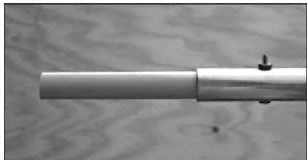
Fig 21.55 — The HVD base insulator is a 1 foot length of 0.75 inch fiberglass rod.
