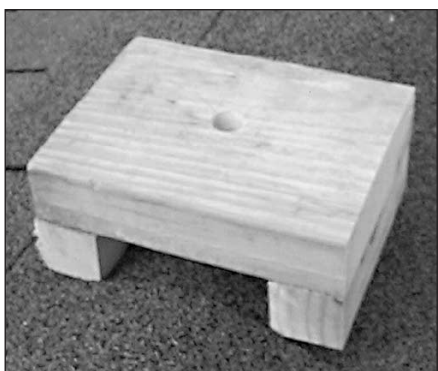
Fig 21.57 — At K8CH, the HVD base insulator sits in this saddle-shaped wooden fixture. This photo was taken before the fixture was painted — a necessary step to protect against the weather.
