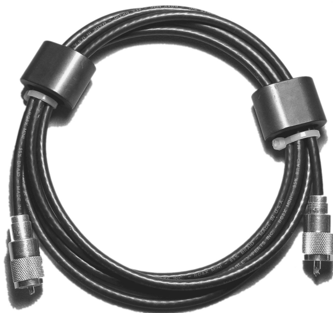
Fig 20.32 — Choke balun that includes both a coiled cable and ferrite beads at each end of the cable.
