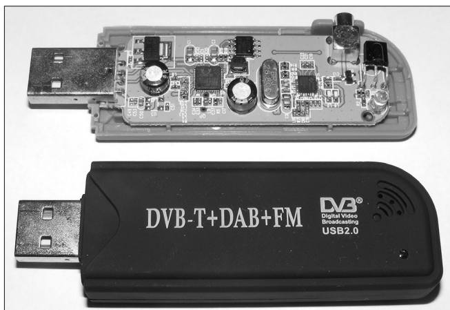
Fig 15.39 — USB dongles containing broadcast TV and FM receivers using the RTL2832U IC.
