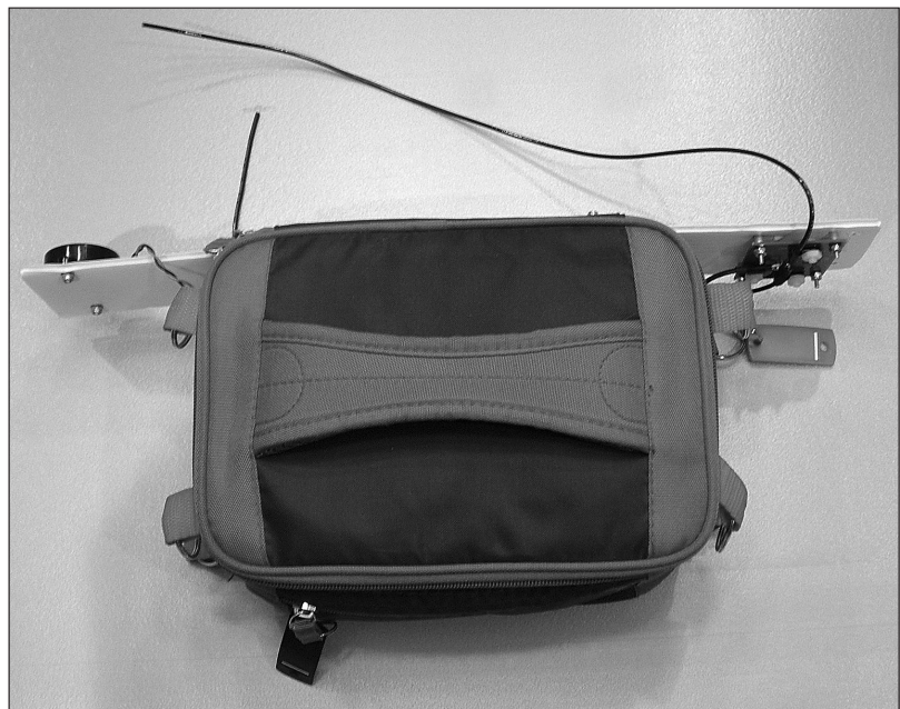
Fig 14.12 — The complete Near Space Tracker assembled in an insulated fabric lunch cooler.
