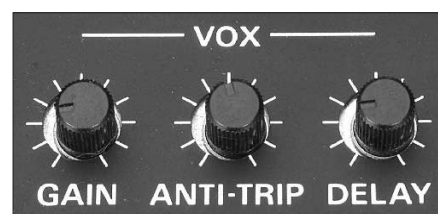
Fig 13.50 — The function of VOX controls is described in the text. They require adjustment for different types of operating, so front-panel knobs make the most convenient control arrangement. In some radios, VOX settings are adjusted through the menu system.
