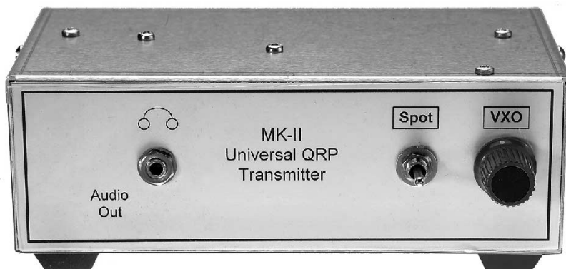
Fig 13.32 — The MKII QRP transmitter includes VXO frequency control, TR switching and a sidetone generator. Construction details may be found on the CD-ROM that accompanies this book.
