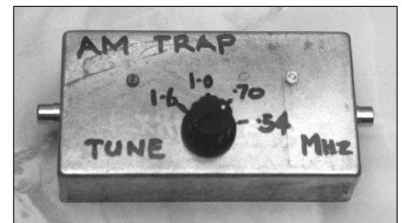
Fig 11.79 — The wave trap can be roughly calibrated to indicate the frequency to which it is tuned.
