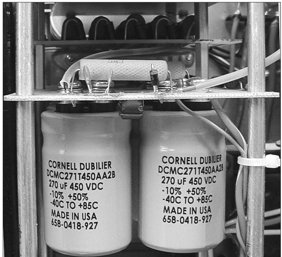
Fig 7.44 — Example of the filter capacitor/bleeder resistor installation in a high voltage power supply.
