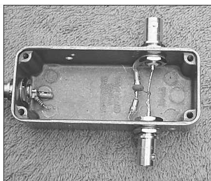
Fig 5.22 — Test fixture for measuring self-resonant frequency of capacitors.
