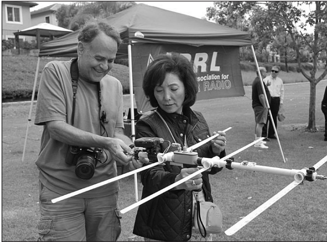
Fig 1.29 — Amateur Radio Direction Finding (ARDF) equipment need not be expensive. Yagis made from measuring tapes and PVC pipe are very popular for direction finding on 2 meters with a handheld transceiver. Here, Dan Slater, AG6HF (left), tests an antenna he built. [Joe Moell, KØOV, photo]
