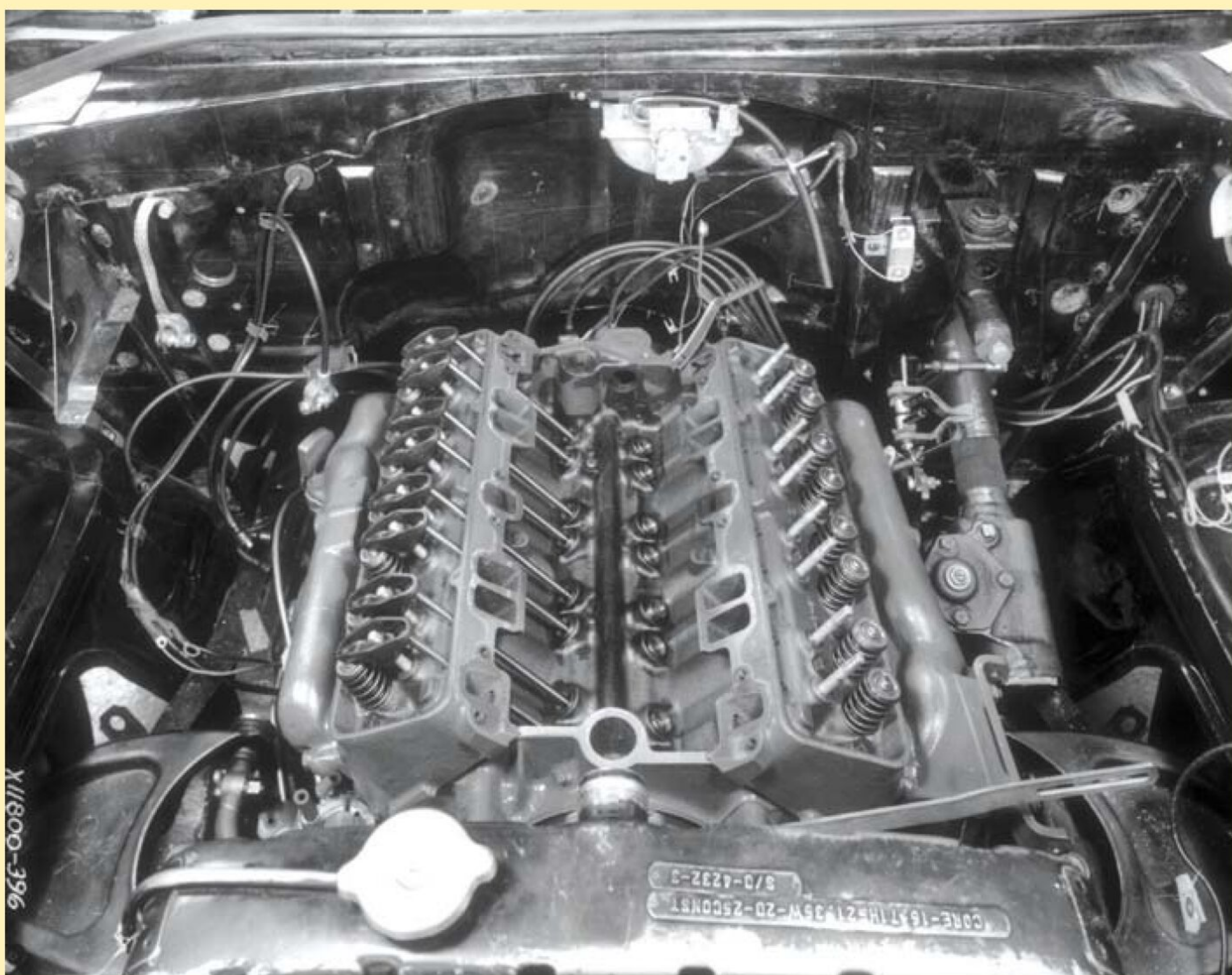
This photo of a prototype Chevy small-block reveals the stamped rocker arms that proved to be a major breakthrough in the design of the engine. (GM Media Archive)
