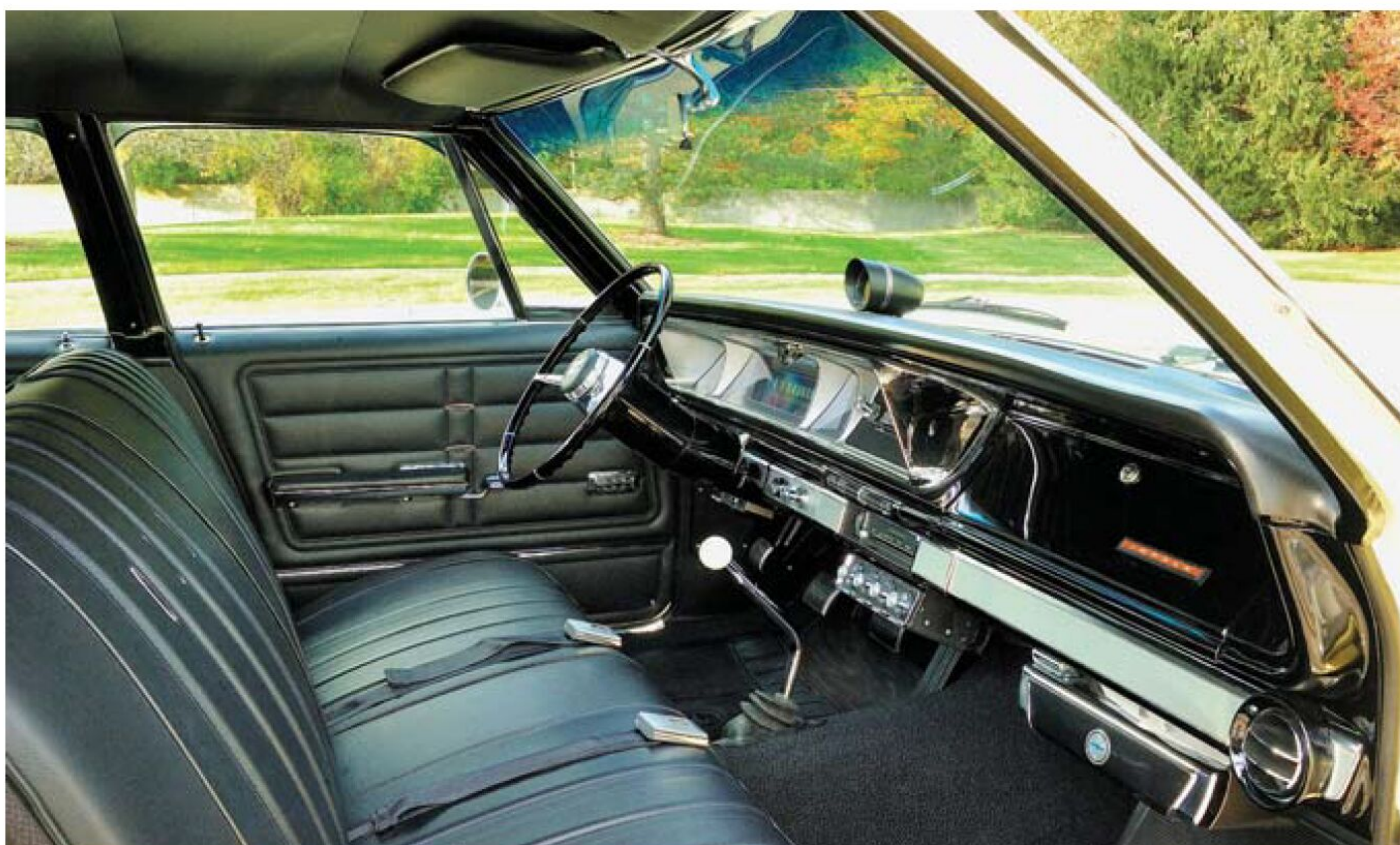
ABOVE: An in-dash tachometer was standard with the 427-engine option, and since the tach was placed in the clock’s location, the clock was relocated to atop the instrument panel.
