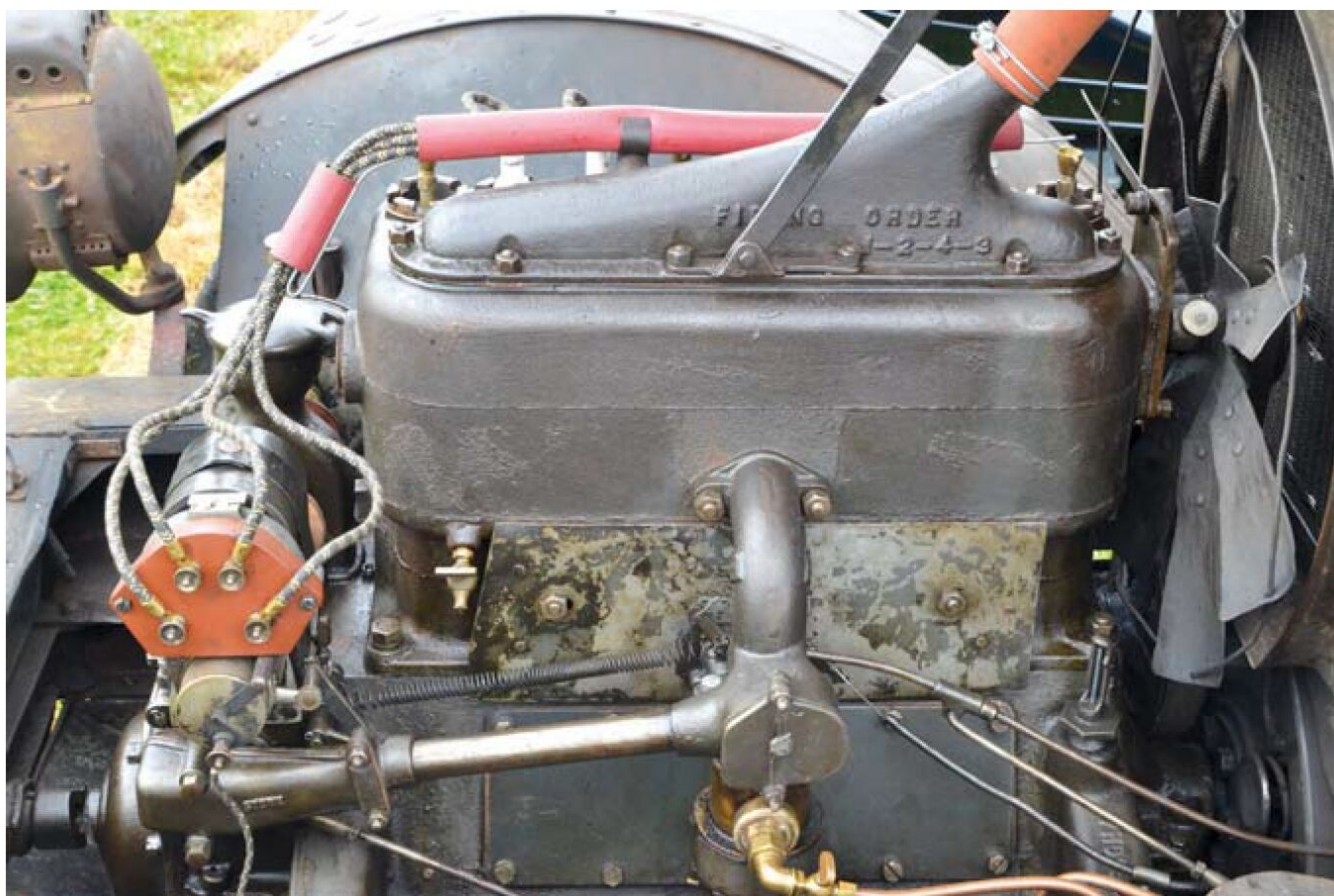
It's difficult to dispute International's claim that the Renault-style hood provides excellent access to the engine. Hiding the radiator behind the engine also prevented damage.
