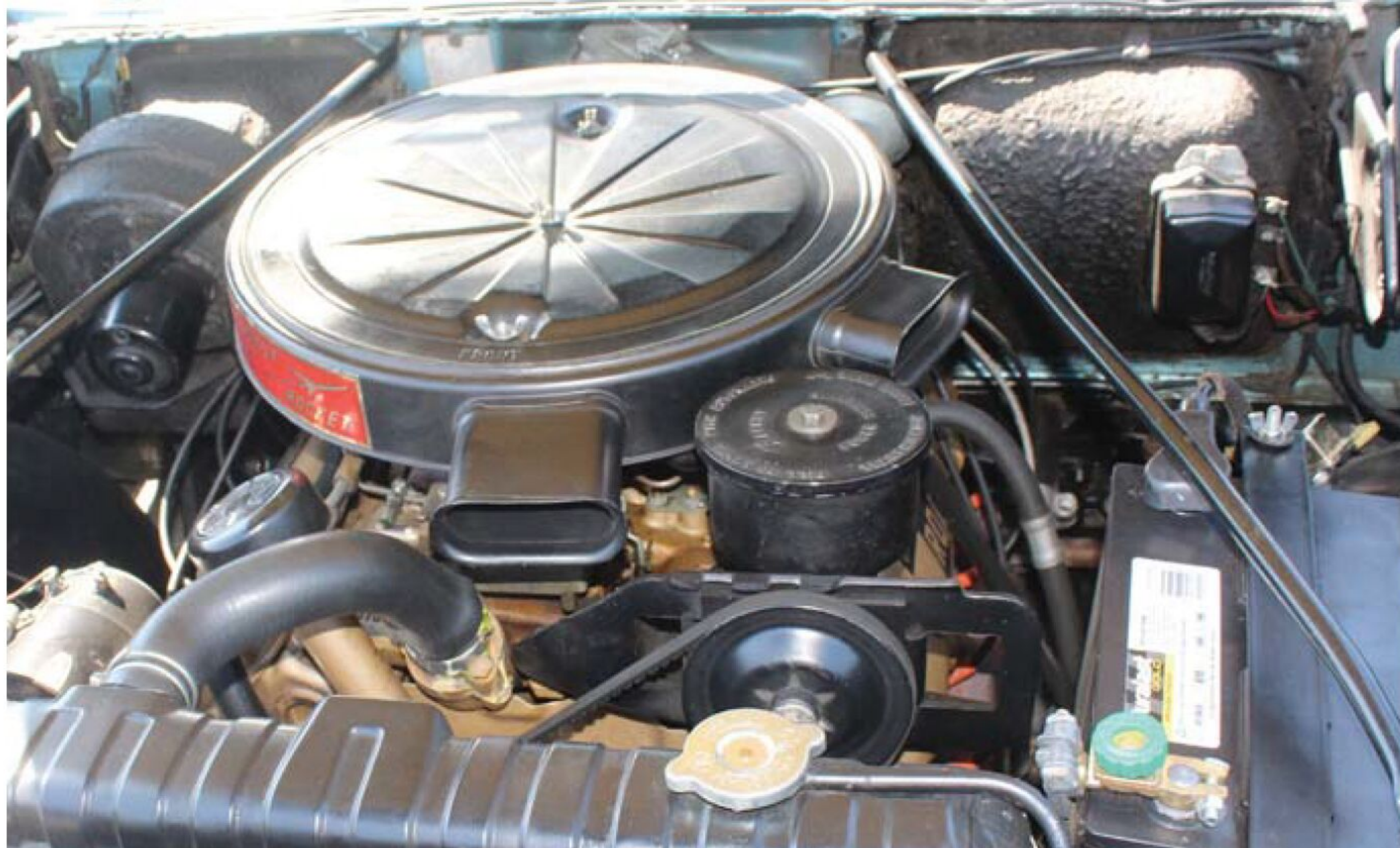
The J-2 option featured three two-barrel carburetors that helped squeeze 312 hp from the 371-cid Rocket V-8.
