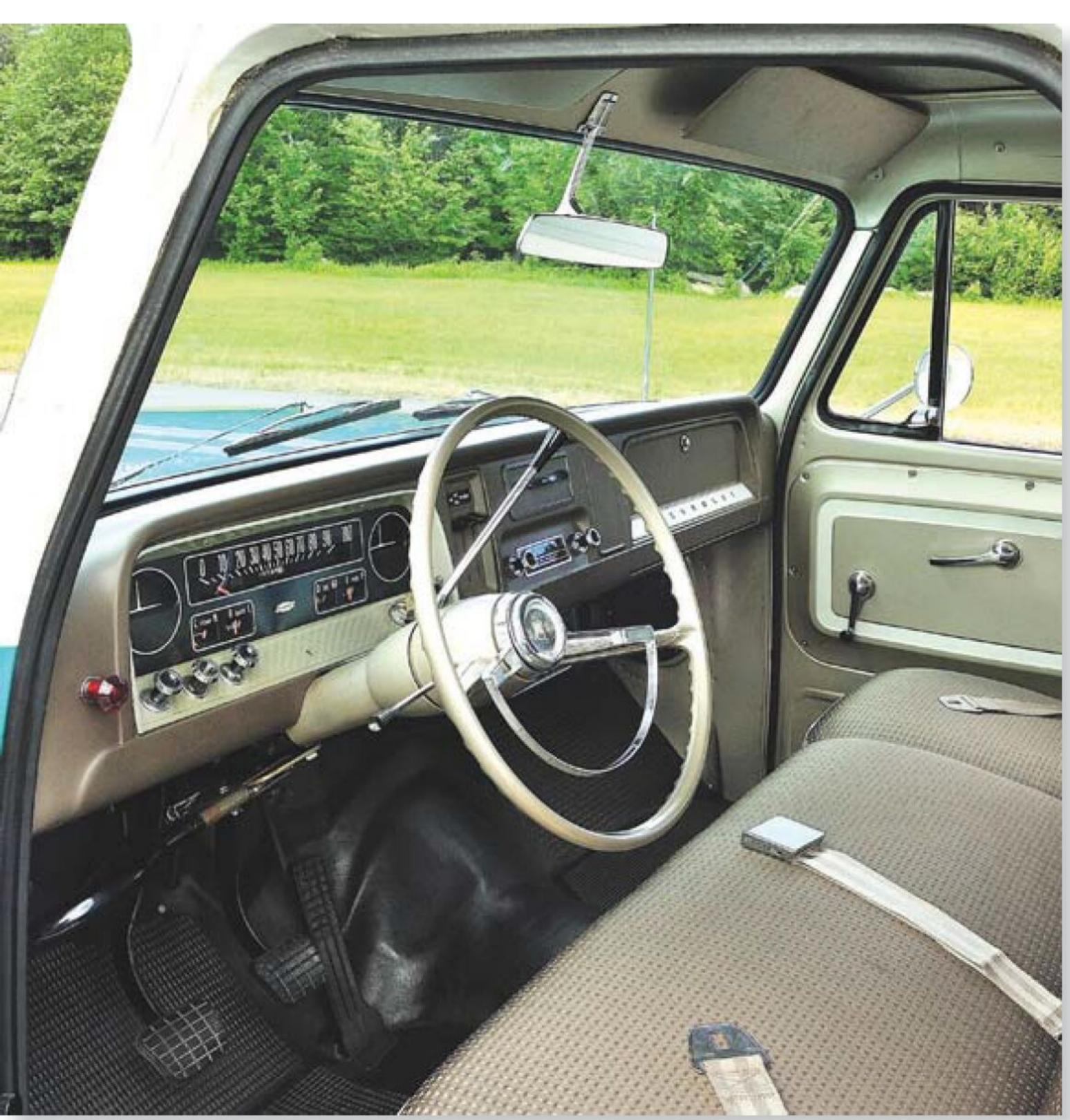
The utilitarian interior was shared with pickup trucks, although the Suburban's front bench seat was split toward the passenger side so the far right side could flip forward for access to the rear seat or seats, depending on whether the truck was built for six or eight passengers.
