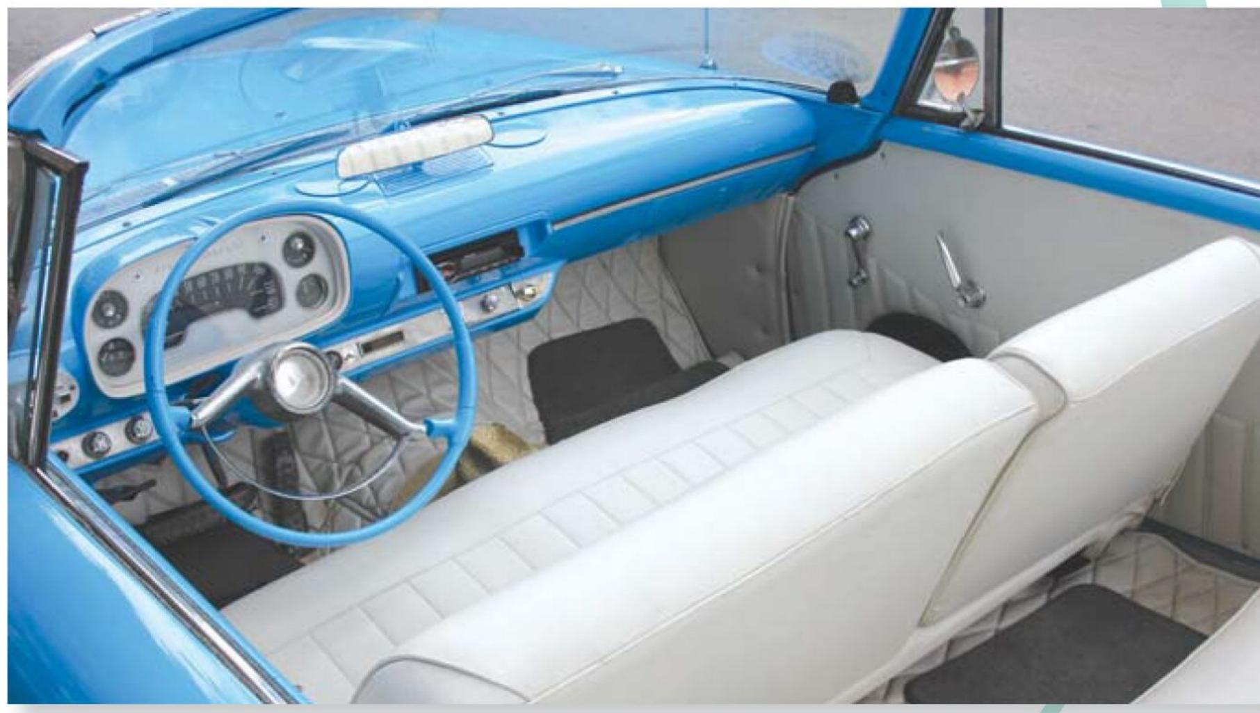
Well-appointed in white vinyl, Hernandez's uncle recently re-upholstered the Plymouth. Note the Plymouth features Chrysler's two-speed push-button PowerFlite transmission console at the driver's left. Chrysler didn't use a locking transmission for the "Park and go" selection in 1957; the cars were placed in neutral and parking brake set.
