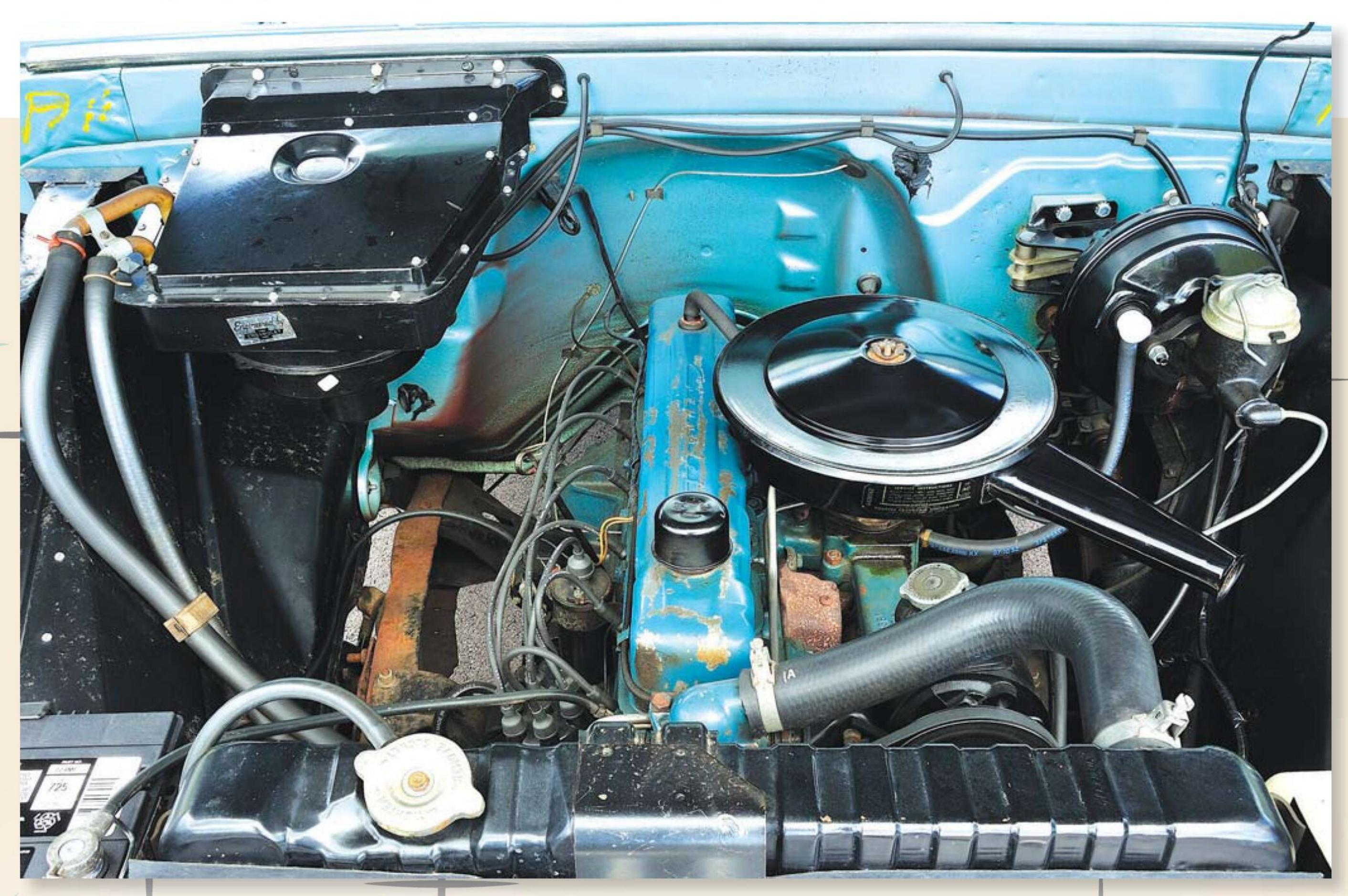
Although optioned with the Custom Comfort Option, this Suburban Carryall was built with the standard 250-cid inline six-cylinder engine, which didn't require a rebuild during its restoration process.
