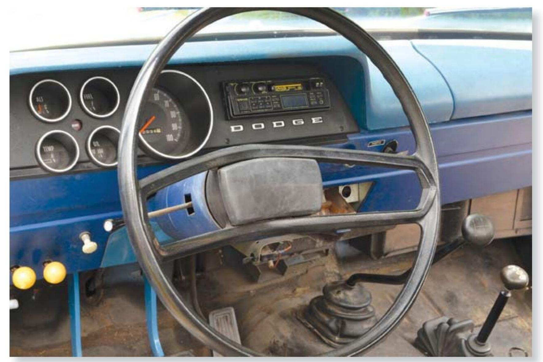
The Dodge's dashboard is an excellent example of the no-nonsense approach to design. The AM-FM-cassette-player replaced the original AM radio, but just inside the steering wheel's right edge is an unusual option: a hand throttle.
