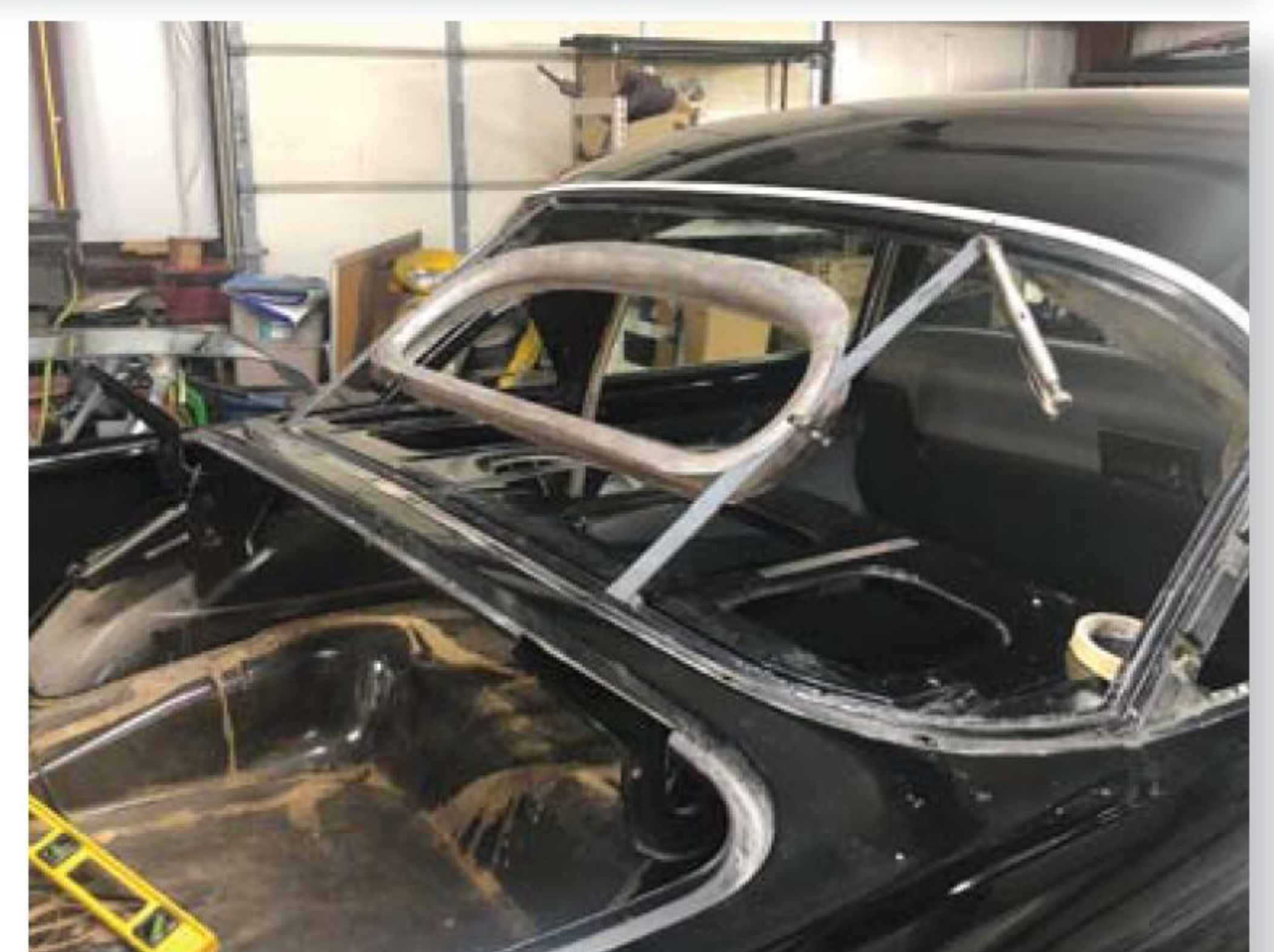
The first step to installing the Derham-style top on the 1956 Premiere was removing the back window and its trim and fitting a new rear window frame.
