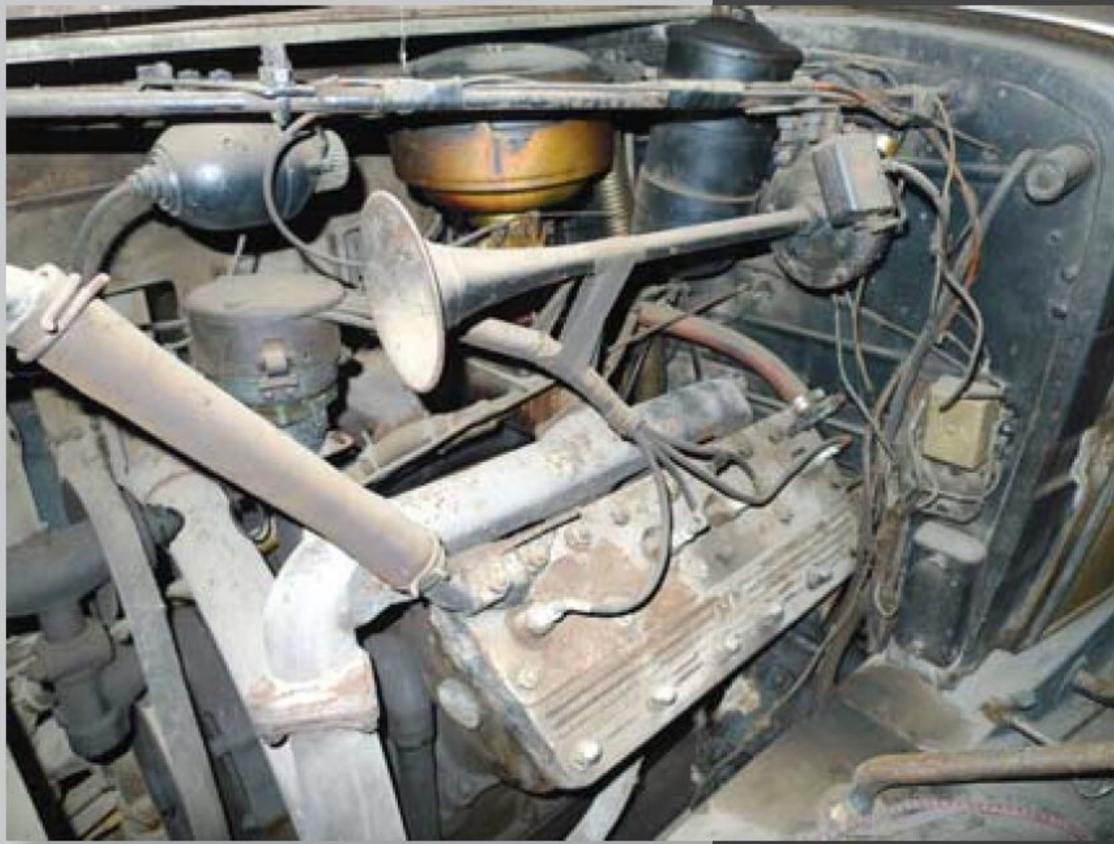
LEFT: V-8 engine displaces 353 cubic inches and appears complete and ready to someday produce its factory 95-hp rating once more.
