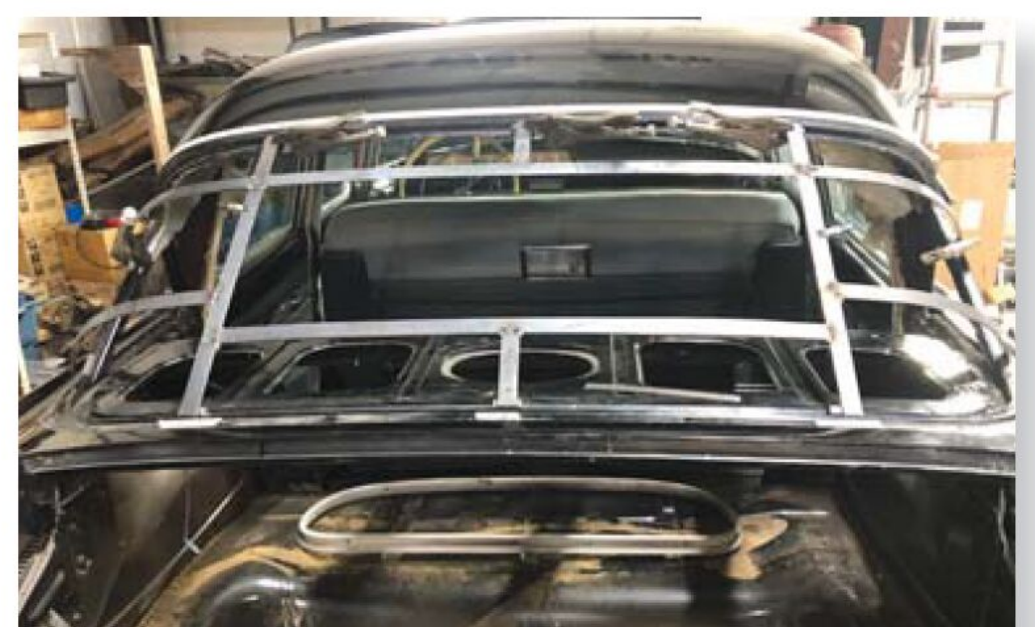
Once the location of the smaller rear window was determined, framework to support the new rear window and padded top could be constructed in the car's original curved rear window opening.
