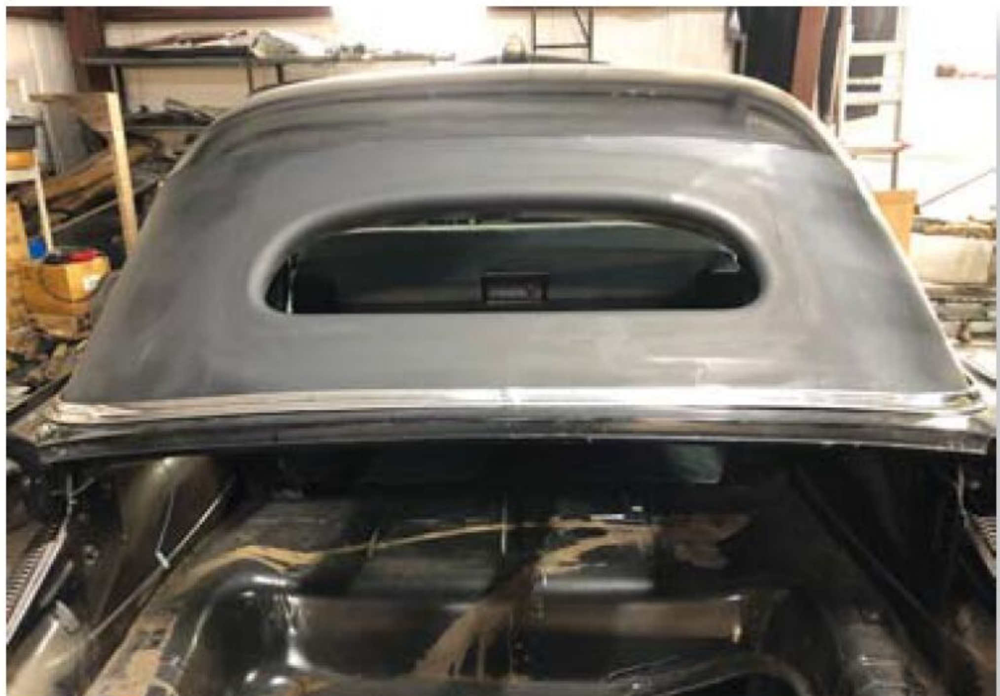
The new metal panels over the framework in the window cavity were made as smooth as the rest of the car's roof in preparation for the padded top.
