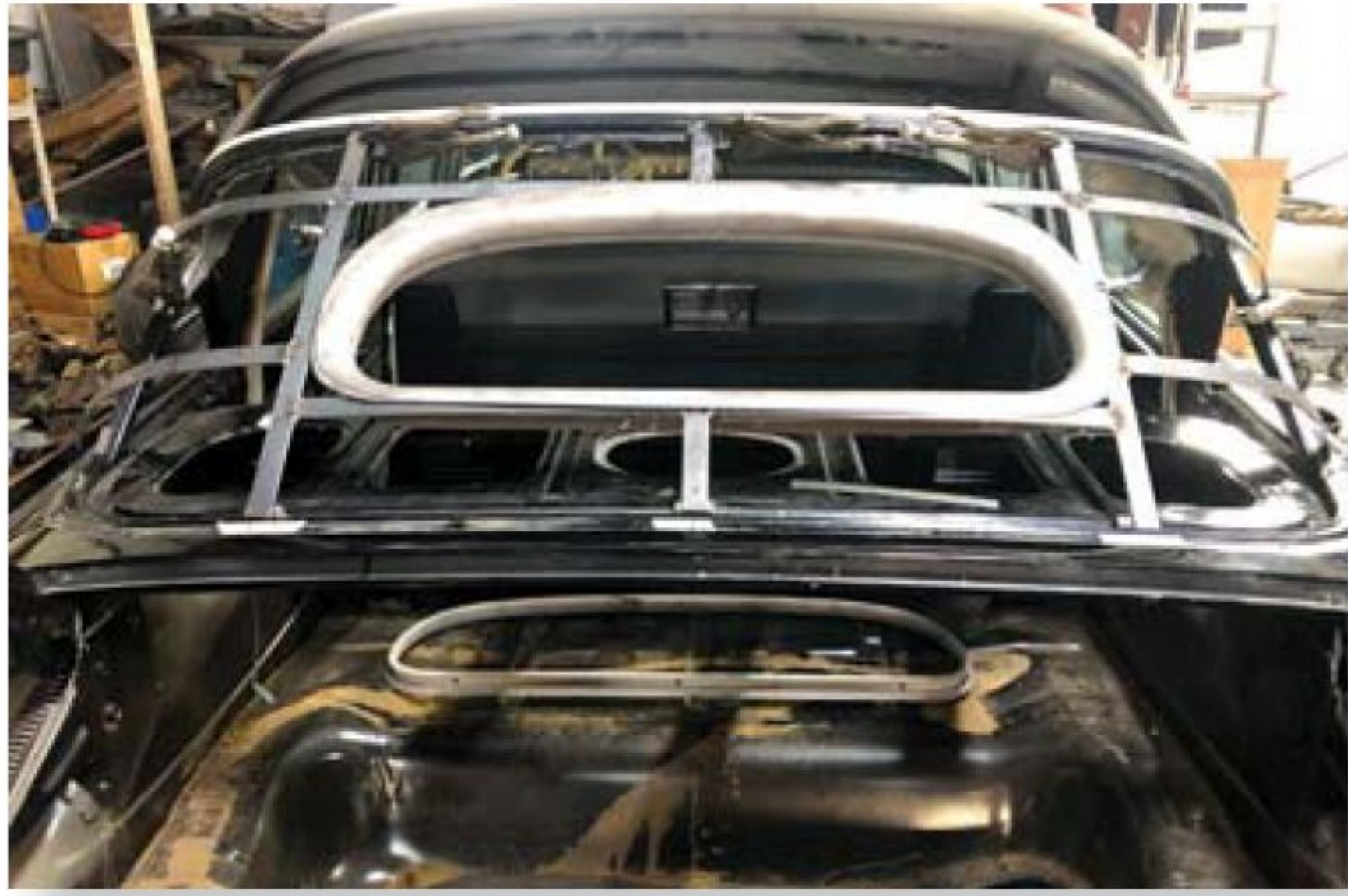
The rear window frame, taken from a 1936 Ford, was nearly identical in size, proportion and shape to rear window frames used by Derham in the 1950s.
