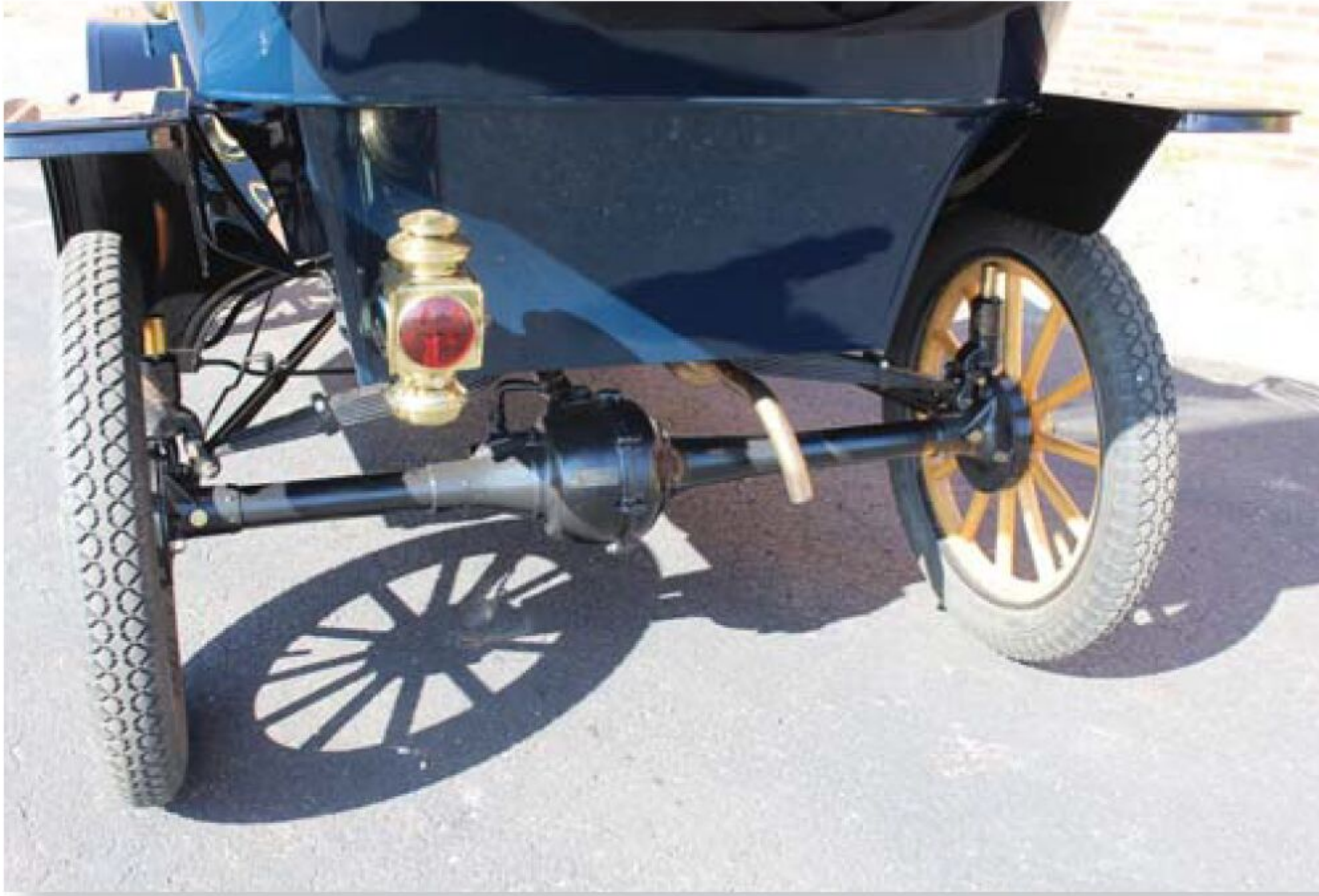
A view from behind shows the Ruxtall two-speed axle that was a popular aftermarket upgrade for Model Ts, along with the K-W Road Smoothers that have been added to help dampen the ride.
