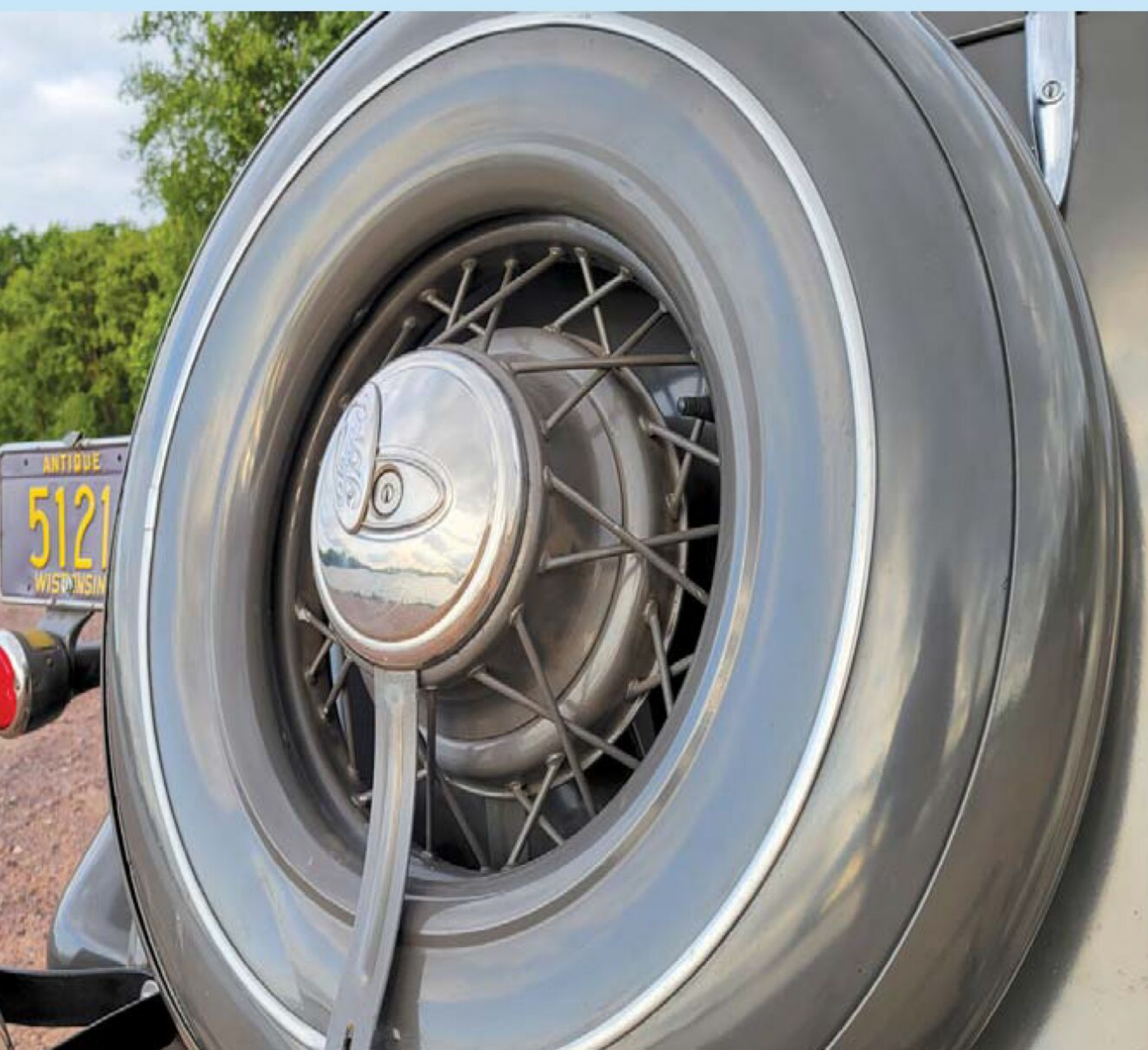
Lock for the rear spare is cleverly hidden behind an oval Ford emblem.
