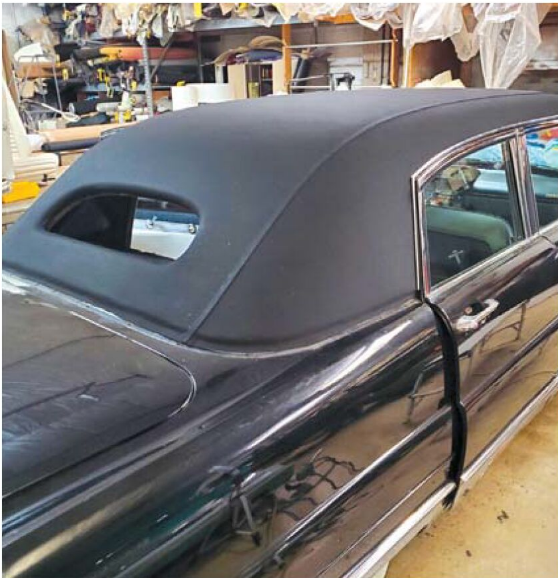
The Landau padding was covered with original-type Stayfast German fabric on the Premiere's roof.
