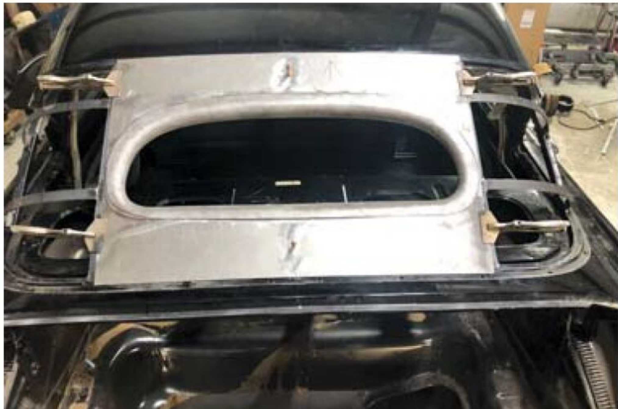
With the window frame in place, metal panels could be affixed to the framework to support the forthcoming padded top.
