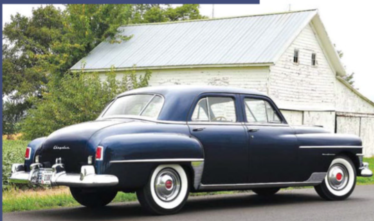
For 1950, Chrysler squared off its cars' rear fenders and lowered the taillamps to the ends of the fenders.
