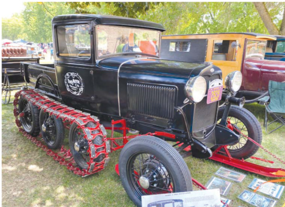
Who says you can't drive old cars in the snow? Steve King's 1931 Ford Model A truck has been fitted with a period Super Snow Bird snowmobile conversion.
