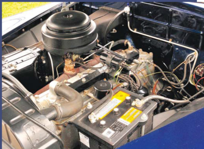
In the last year for Chrysler's straight-eight engine, it produced 135 bhp and had 270 lb.-ft. of torque.
