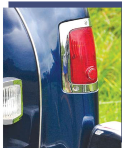
Taillamps were moved to the rear of the more squared-off 1950 Chrysler fenders, which added a greater look of length.
