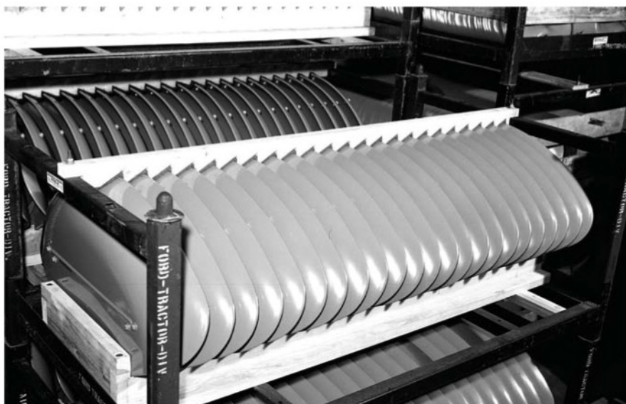
Parts for tractors were shipped to the factory pre-painted and ready for installation, as shown by these fenders for the 2N tractor.
