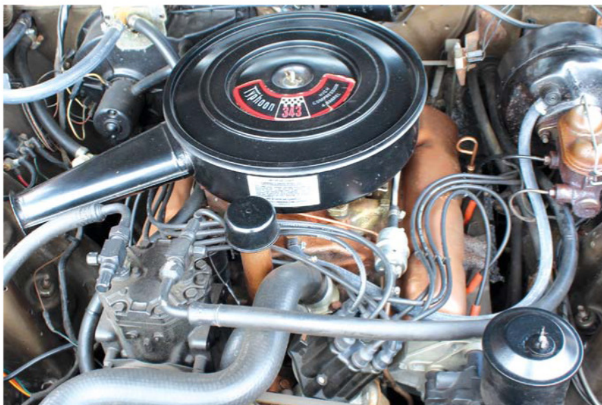
The “Typhoon 343” with a four-barrel carburetor was at the top of the engine option list in 1967. It produced a more-than-respectable 280 hp from 343 cubic inches.
