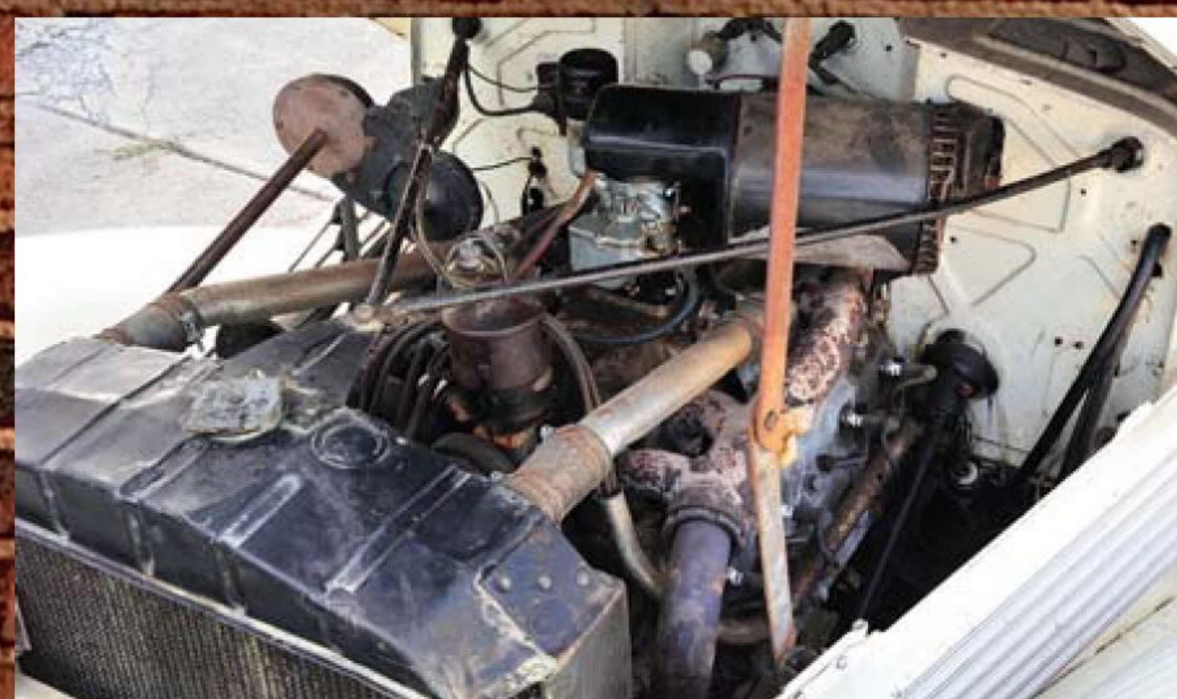
The 1936 and 1937 Cords were driven by a flathead V-8 displacing 288.6 cubic inches with a transmission mounted in front of the engine.
