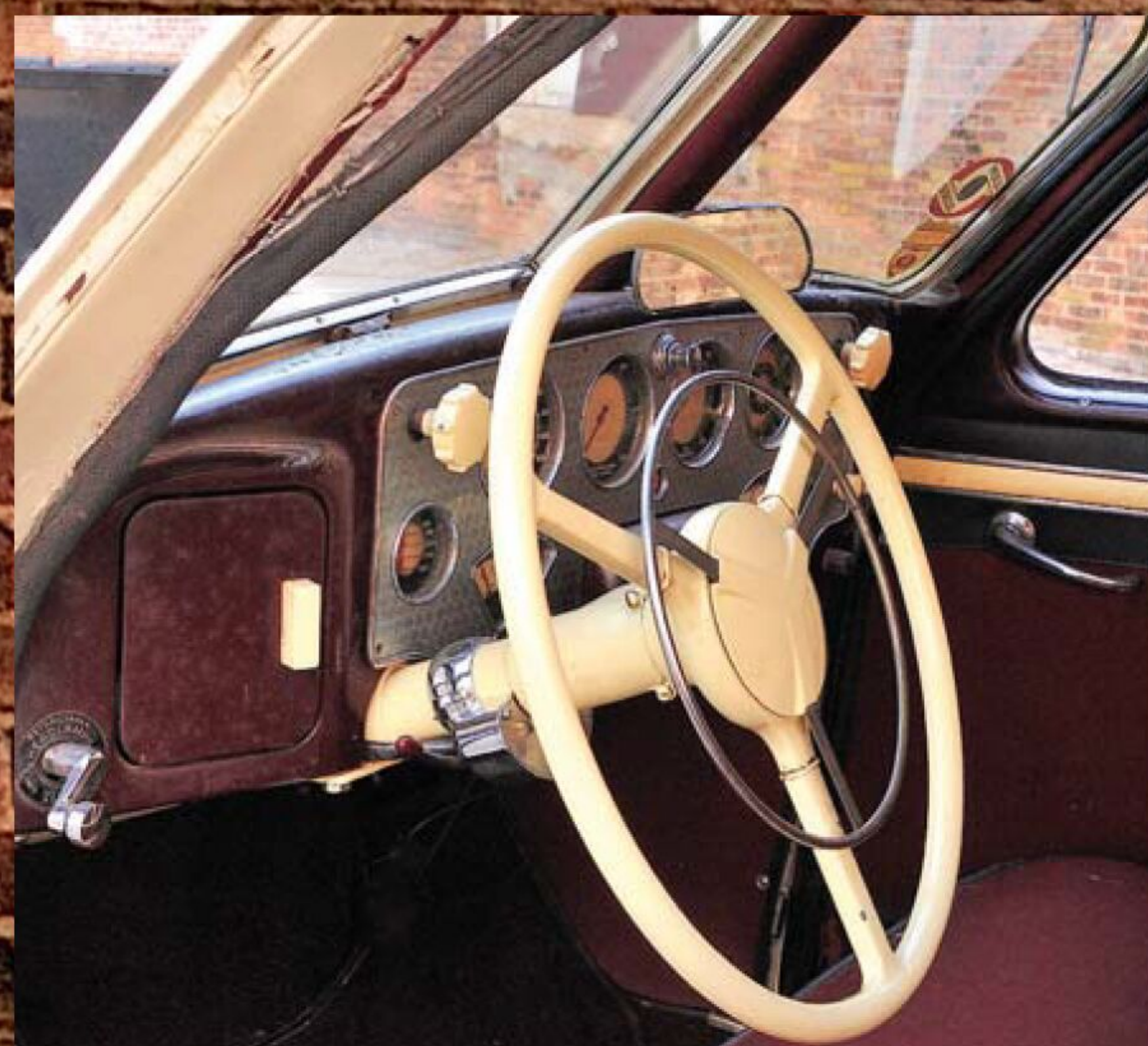
John Pontius thinks the Cord was restored in the 1970s at which point seat covers were placed over the original upholstery. The crank at far left mechanically raises the Cord's headlamps.
