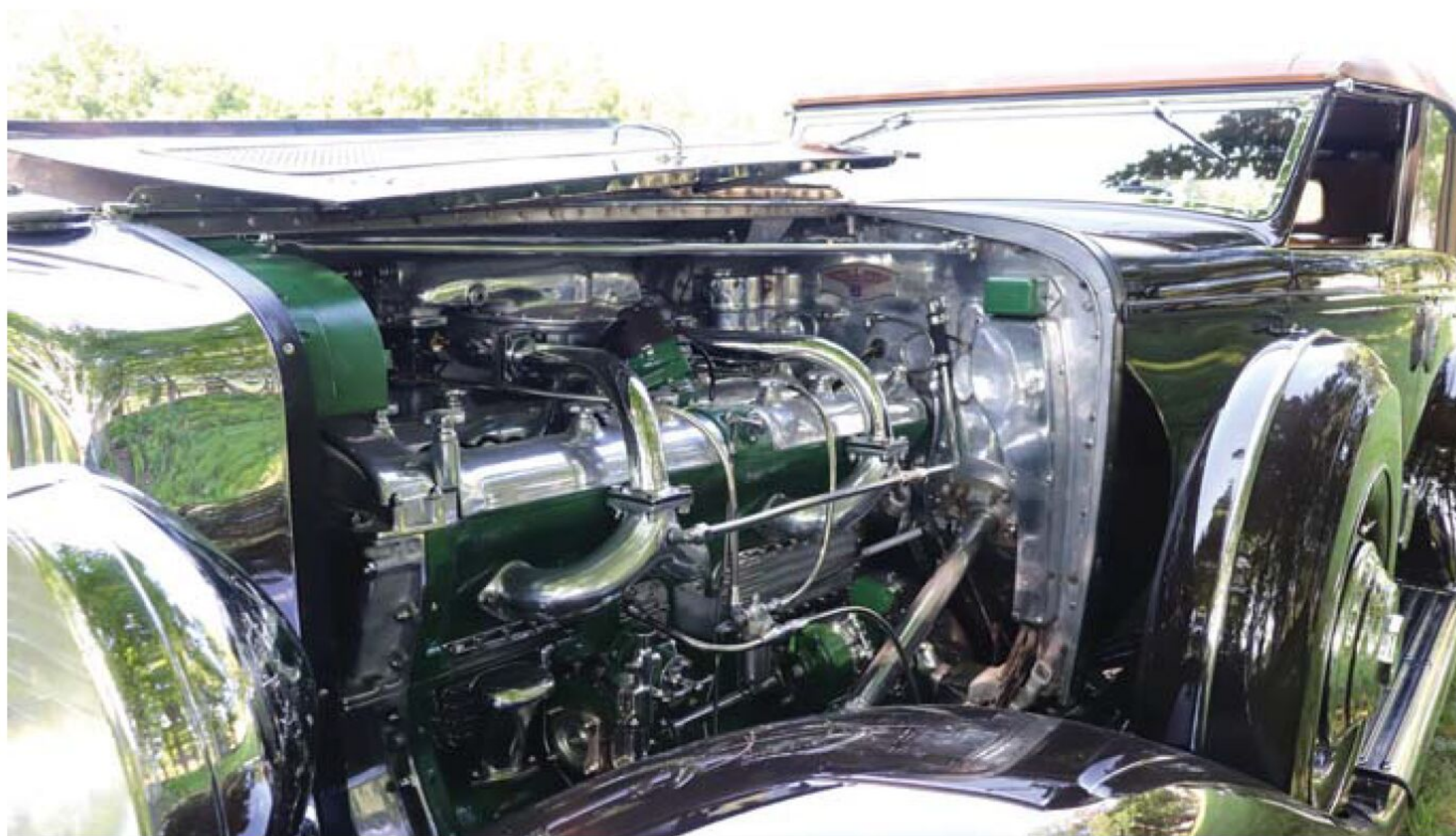
The dual carburetor setup includes ram's horn manifolds that cross over the top of the engine.
