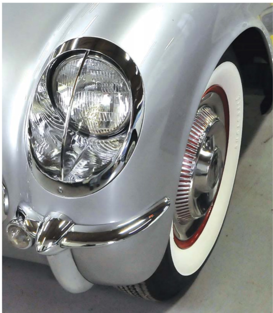
BELOW: The blades over the headlamps are unique to this Corvette. Note how they line up with the vertical part of the bumperette and almost appear as an extension of them.
