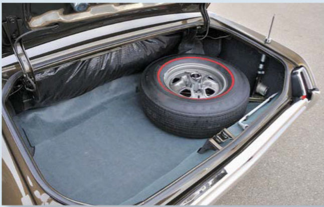
The trunk holds a fifth Super Stock II wheel and the base for the optional power antenna; the deck lid has the optional power release.
