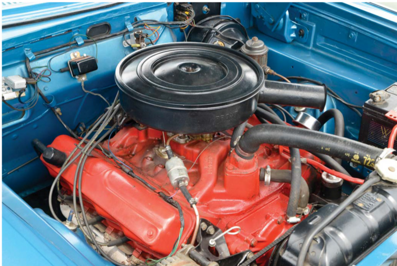
The Sport Fury's base engine in 1962 was the 318-cid V-8 with its 230 hp. The engine shown here is a rebuild that came from a parts car to replace the seized original.
