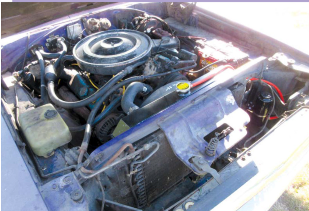
In 1970, the Dodge Charger could be equipped with a six-cylinder or a 318-cid. V-8, but this Charger was originally powered by the optional 383-cid V-8. The original 383 of this Charger was replaced after an oiling issue.
