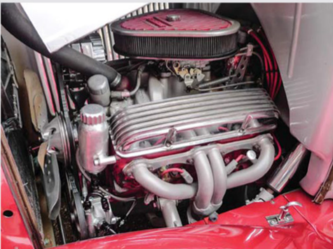
The current Chevy mill is a 350-hp, 350-cid LT1 with machine work by Wayne's Engine and assembled by Henry. Block-huggin' headers are by Henry as well.
