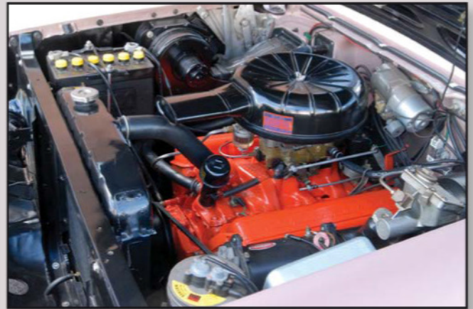
Chevy's modern V-8 was in its third year in 1957, and its descendants would be built for decades. As a group, they would be known simply as "small blocks."
