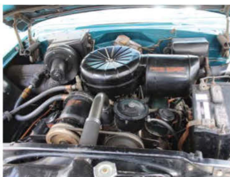
Safari motivation for 1956 originally came from a 316.6-cid V-8 that pushed out 216 hp with the three-speed or 227 hp with the Hydra-Matic automatic. This engine is a 347-cid V-8 transplant from a 1957 Pontiac, but Miller still has the original 316.6-cid power plant. At right: The clamshell-style tailgate has a lot of moving parts, but was there ever a cargo area that looked better than this?
