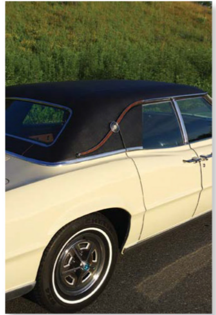
Above: The C pillar was cleverly integrated into the rear doors of Thunderbird four-doors and maintained rear-seat privacy while also aiding entry and egress.
