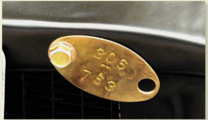
A reproduction of the original brass tag indicating the Mustang was initially a Ford Motor Co. test vehicle was mounted on the Mustang's radiator support.
