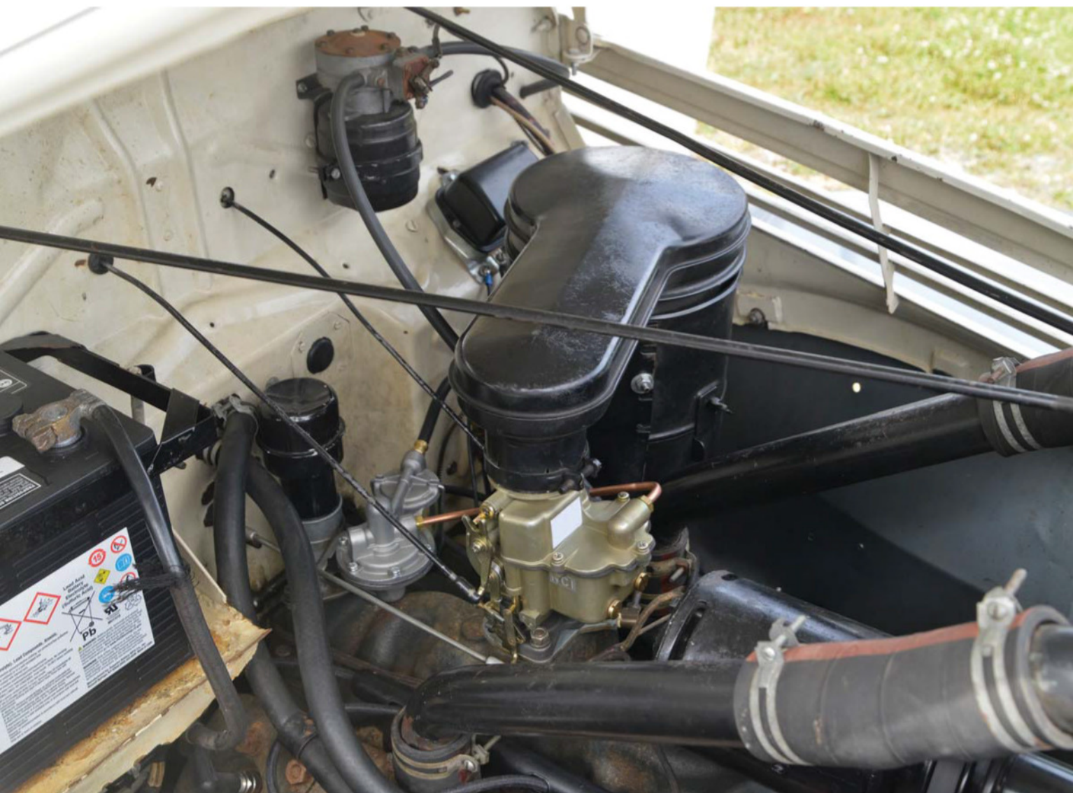
By 1939, Ford's Flathead V-8 was a proven design that retained the aura that surrounded it at its introduction. It displaced 221 cubic inches in 1939.
