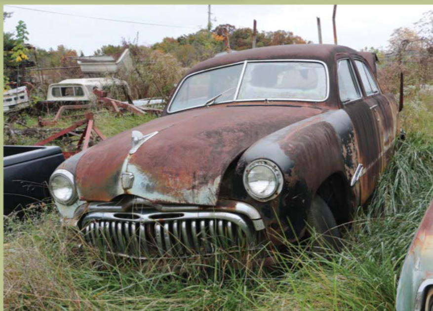
Ill-fitting and crooked Buick teeth do nothing to improve the looks of this 1951 Ford. The hood appears to be from an earlier 1949 or '50 Ford,
