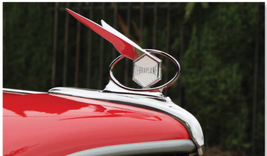
The Terraplane hood ornament consists of the traditional Hudson hexagon within an oval topped off by two wings.
