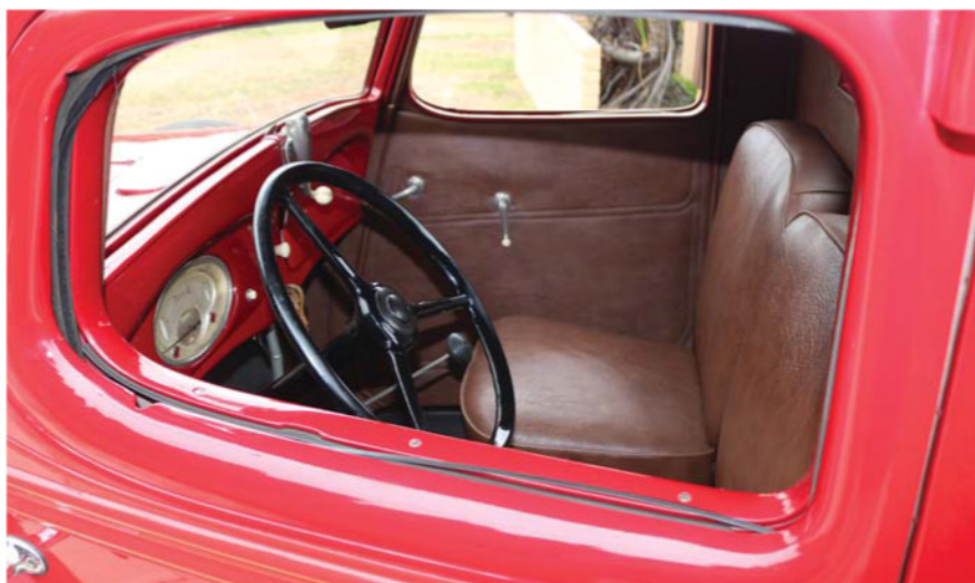
Interiors of 1930s trucks are generally Spartan, and the Terraplane is no different with its single instrument cluster and monocolour upholstery, which lacks armrests on the door panels.
