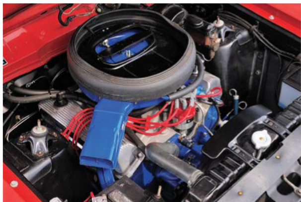
Above: The Super Cobra Jet 428-cid V-8 was good for 335 hp in 1969, but this one has some internal tweaks to bump up the “h-p.”
