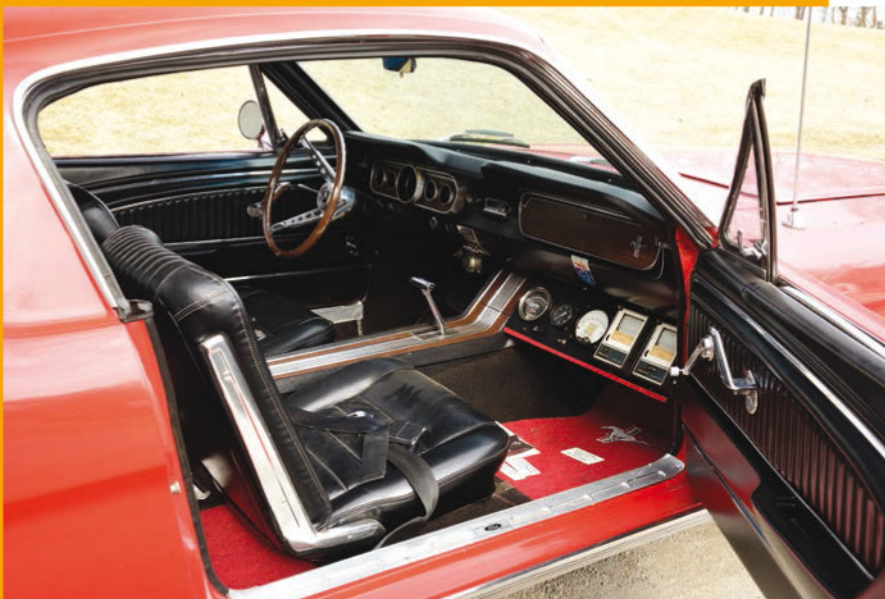
A series of gauges were mounted below the instrument panel to monitor the rotary engine's functions during testing.
