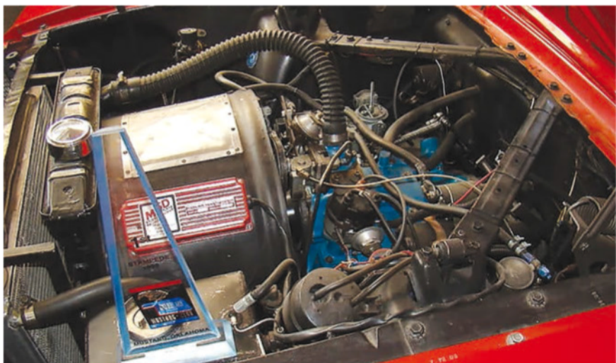
The rotary engine in the engine compartment of the 1965 Mustang. It has since been pulled from the Mustang for a rebuild that has stalled.
