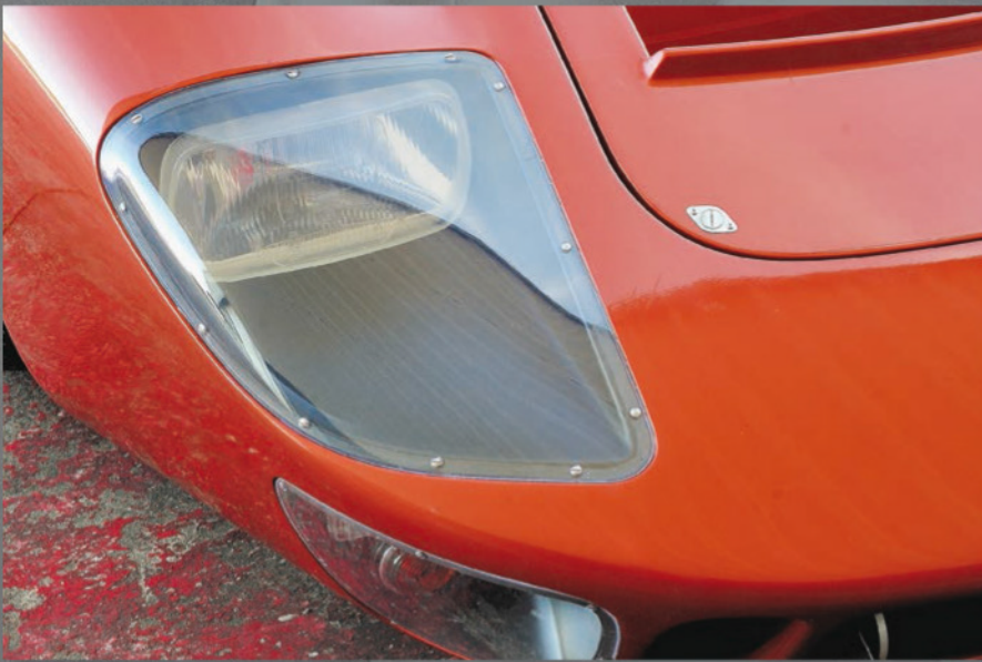
Headlamp covers improve aerodynamics and shield the bulb from debris when racing.
