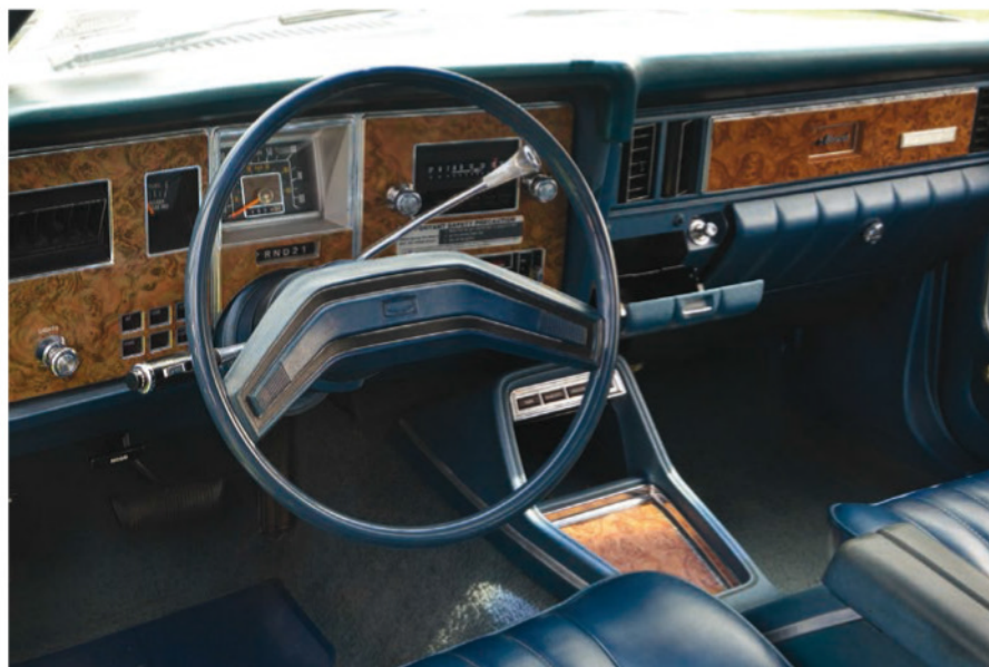
An 85-mph speedometer and the "important safety precautions" decal below the Aeronutronic AM radio. The Monarch S option group included the bucket seats.
