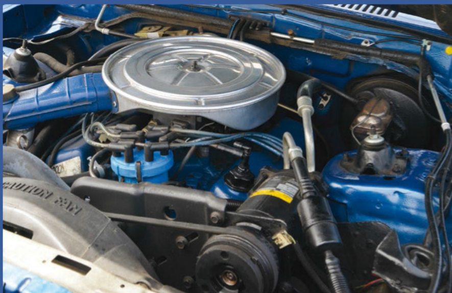
The Monarch's 302-cubic-inch V-8 was rated at up to 137 hp as early emissions-control equipment was taking its toll. That number probably wasn't as bad as it seemed at the time since it was a net figure, which is automatically lower than the gross horsepower rating used throughout the industry until just a few years earlier.
