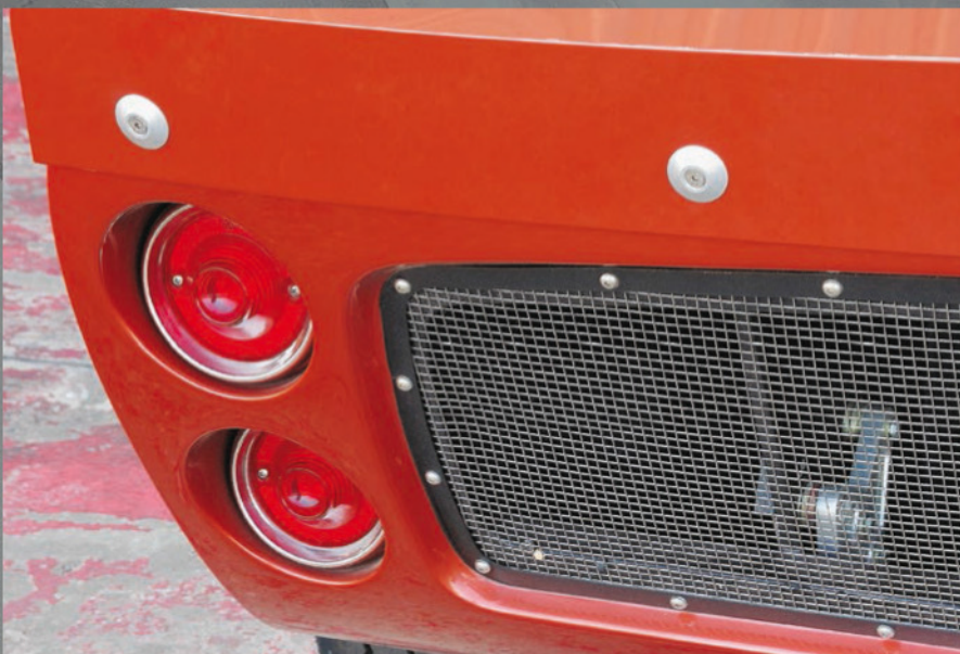
Designed by Ford racing legend Dan Gurney, the "Gurney Flap" mounted horizontally across the rear of the GT40 is designed to force air downward for improved handling.
