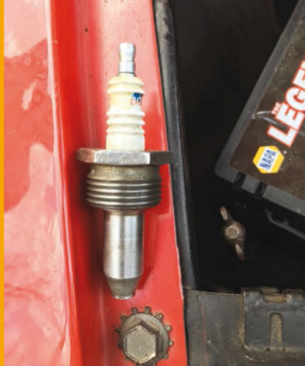
The unique spark plug used in the rotary engine is a Champion unit marked "365-4."
