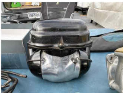
This Berk conversion of a Lincoln-Zephyr dual-point/dual-coil distributor would take a Ford or Mercury V-8 to more than 5,000 rpm. Spaulding built a similar conversion. If you want one, they are $750-$1,000.
