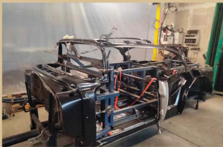
Construction of the new body for the recreation 50 Millionth GM car underway at Real Deal Steel.
