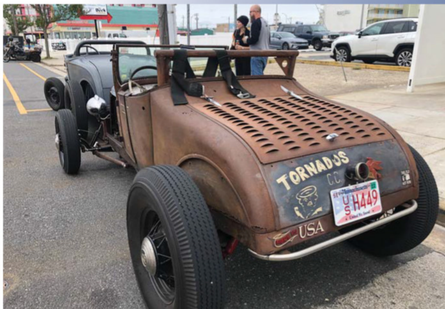
This '27 T from the Tornados Car Club in Massachusetts has a square roll bar. Whatever rollover protection these might have provided was negated by the angled ends, which had a tendency to dig into the ground when a car flipped. But they look cool, right? KEN GROSS PHOTO
