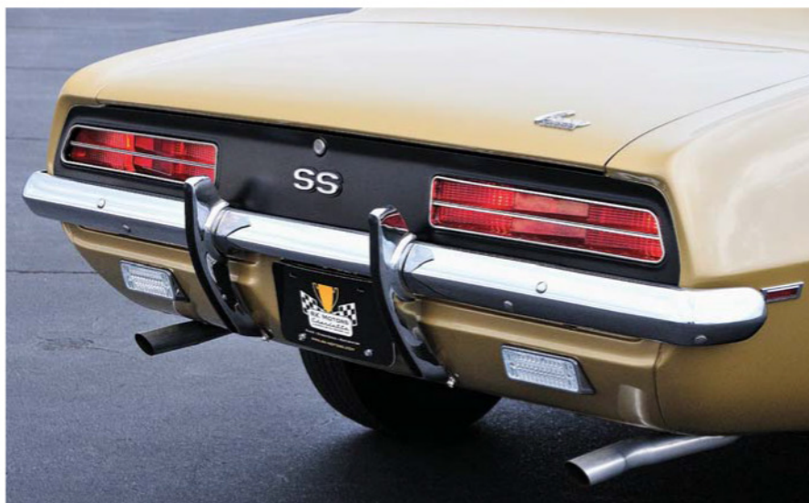
The tail panel of Camaro Super Sports with the 396-cid big-block was painted black, except on pace car models. The unique Rally Sport "triple-unit taillights" lacked a back-up lamp, so RS models received separate back-up lamps beneath the bumper.
