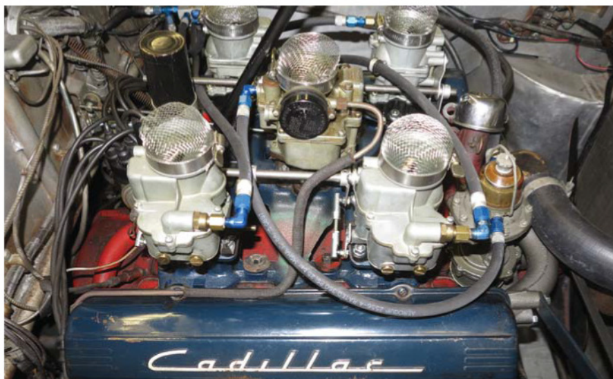
A quartet of Holley carburetors encircle the central Carter carburetor on the unique manifold fitted to the 331-cid V-8 of the “Le Monstre” roadster. Unfortunately, the coupe has lost its unique dual two-barrel carburetor setup since the race.
