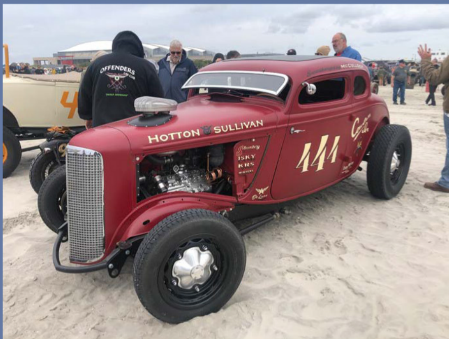
This hard-chopped '34 five-window had everyone talking. It's powered by a big stroker Flathead with Hotton & Sullivan high-compression heads and a McCulloch centrifugal supercharger, topped by twin Strombergs. Don't you love that Cadillac grille and the alloy caps on "wide 5" wheels? KEN GROSS PHOTO
