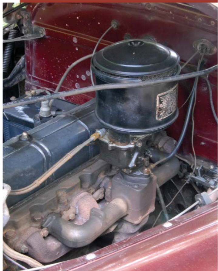
Under the hood is the ever-reliable Chevy six. Its 216 cubic inches provide 90 hp, an increase from 85 a year earlier.
