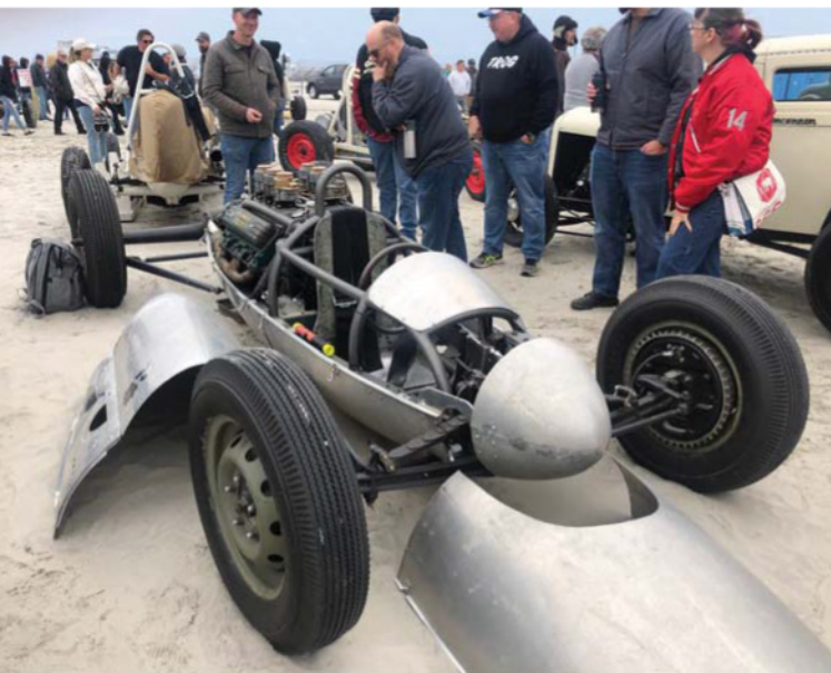
One of the potentially quickest cars was this Olds-powered belly tank with a six-carb log manifold. It's scary, but the Buick finned drums would help it stop. Somewhere, Tom Beatty is smiling.
