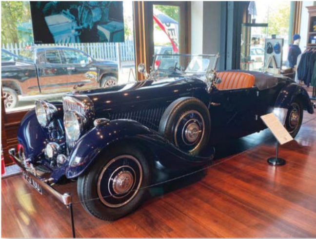
A 1937 Bentley powered by a Rolls-Royce 4-1/2-litre engine with coachwork by Carlton Carriage Co. This was Bentley's only two-seat open touring car of the period.
