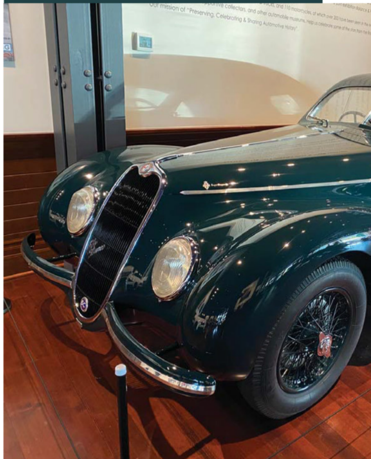
1939 Alfa Romeo was one of Italy's greatest grand touring cars of the 1930s and featured an all-aluminum body.
