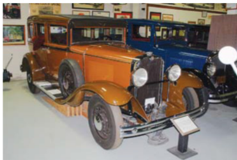
From 1930 to 1931, Oldsmobile had a companion model, the Viking. Shown is a 1930 Viking sedan. While Oldsmobiles were powered with a six-cylinder engine, the more upscale Viking was powered by a 90-degree V-8.
