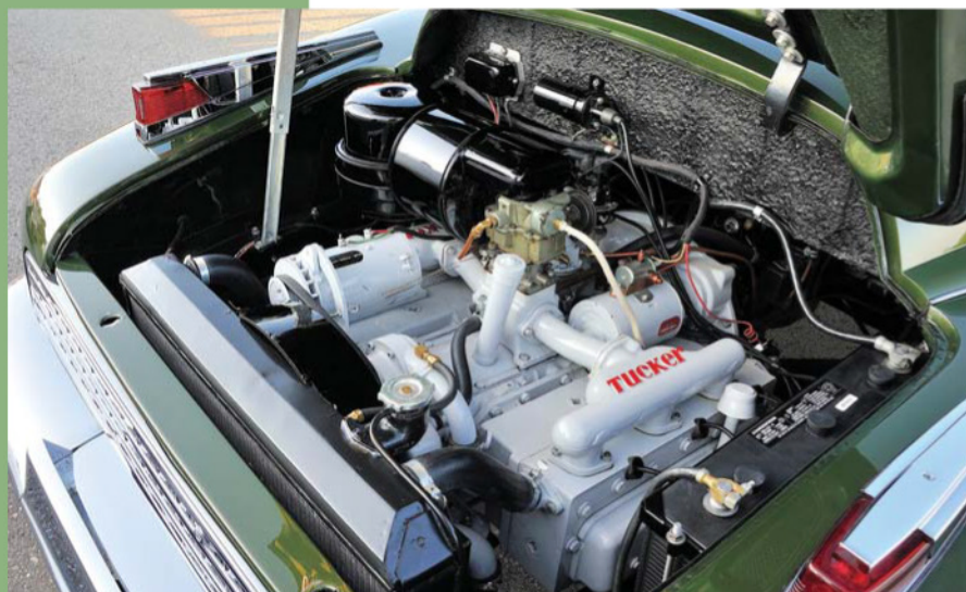
The Tucker's six-cylinder, water-cooled, horizontally opposed engine was originally developed for a helicopter application.
