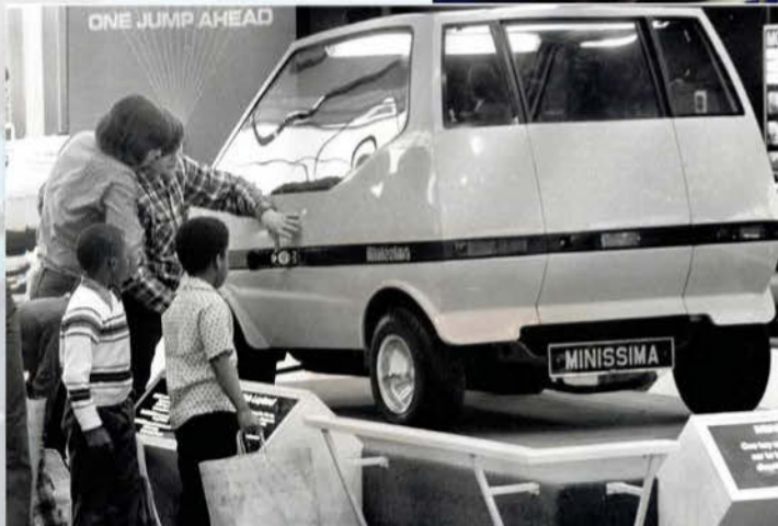
Minissima, a little experimental commuter car from British Leyland Motors, was fitted with a 38-hp engine claiming 40 mph.
