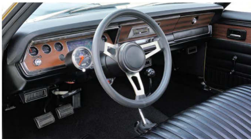
The four-speed manual transmission and Tuff steering wheel were part of the Rallye package, and the woodgrain interior trim was part of the Sport package. As part of its “day two” upgrades, the Dart has a column-mounted aftermarket tachometer like so many of its contemporaries.
