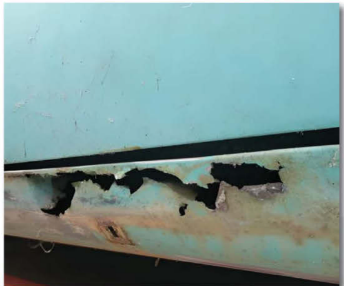
This rocker is far from rockin'! Time to cut out the cancer and replace it with fresh sheet metal. If you are from the North, this is a common sight among our "seasoned" old cars stock.
