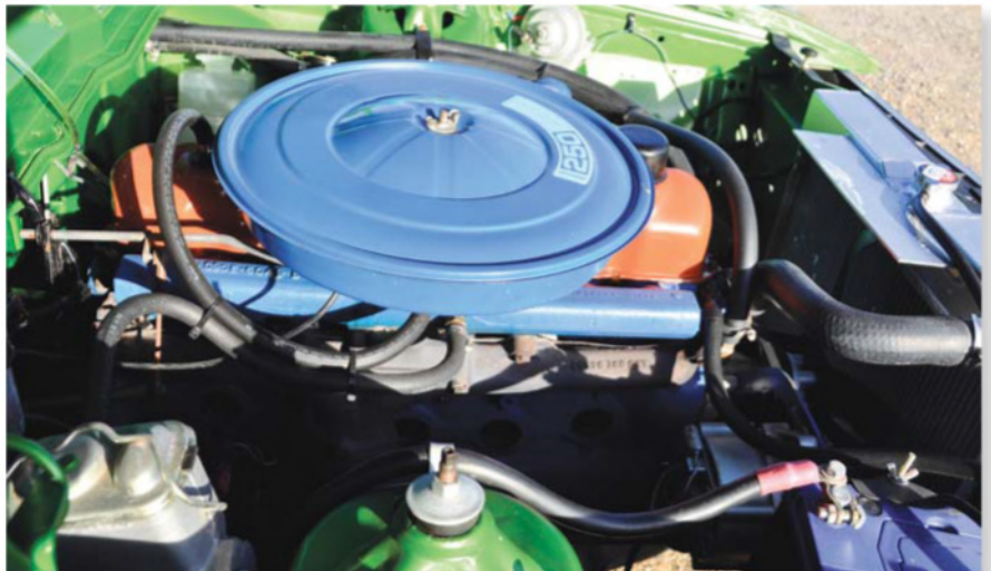
Engine bay with the original 250-cid six-cylinder power plant.
