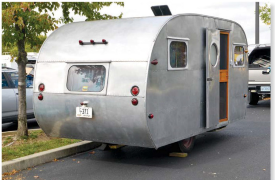
Rounded rather than streamlined, this 1955 Zollinger Va-Ka-Shun-Ette had suffered water damage before its current owner bought it and replaced several of its aluminum panels.
