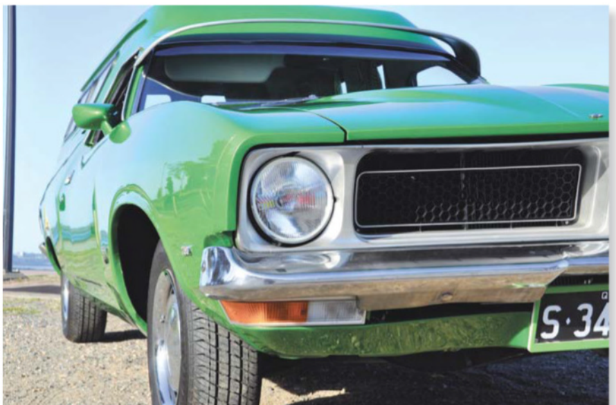
Falcon XB headlamp bezel is reminiscent of the 1966 Studebaker while grille has shades of the Plymouth Barracuda; note its honeycomb grille texture.
