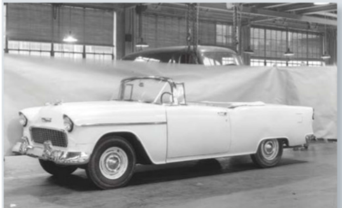
This Fisher Body-built convertible was used for testing at GM's Milford, Mich., proving grounds. Early cars such as this one were not fully trimmed, but had all major hardware installed. Note parking lamp openings were covered with plates. (GM Media Archive)
