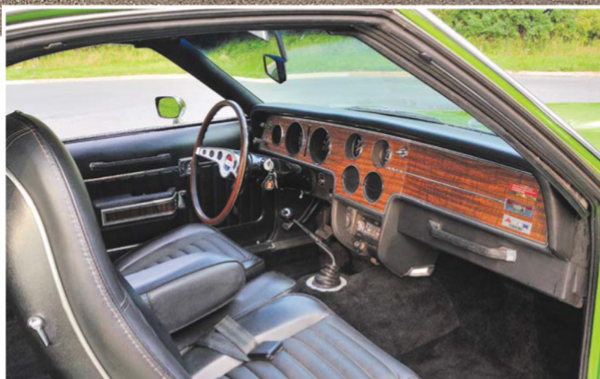
The fully synchronized four-speed manual transmission and vinyl bucket seats were no-charge on the 1970 AMX, as was the instrument panel with a tachometer and sports steering wheel.
