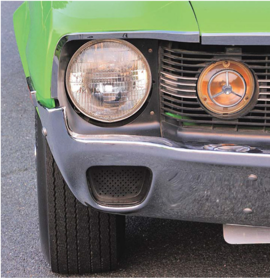
For 1970, the parking lamps/turn signals were moved from the bumper to the grille of the AMX, giving the muscle car a more menacing look.
