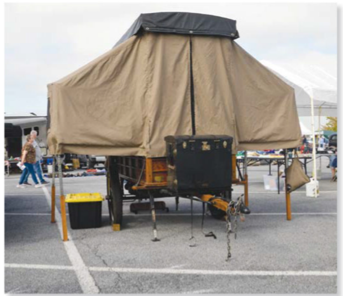
Built to participate in a 2019 tour, this popup resembles a Model T Ford depot hack because that provided some of the dimensions and patterns used in its construction. A 1914 Model T is its regular tow vehicle.
