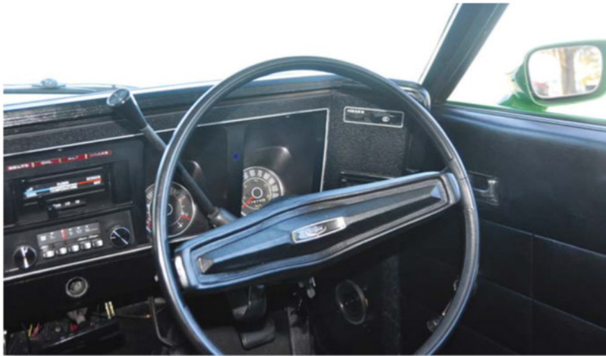
Instrument cluster curves around in front of driver. The steering wheel is on the right side.
