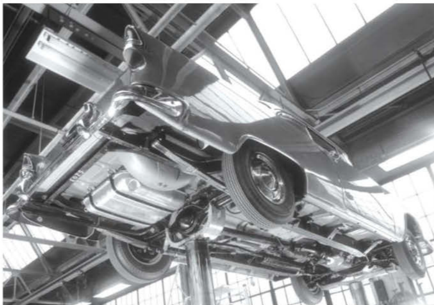
Test car 5203 (note stencil on rear frame cross member) was thoroughly photographed inside the GM Proving Grounds garage prior to the car's 25,000-mile test run.
