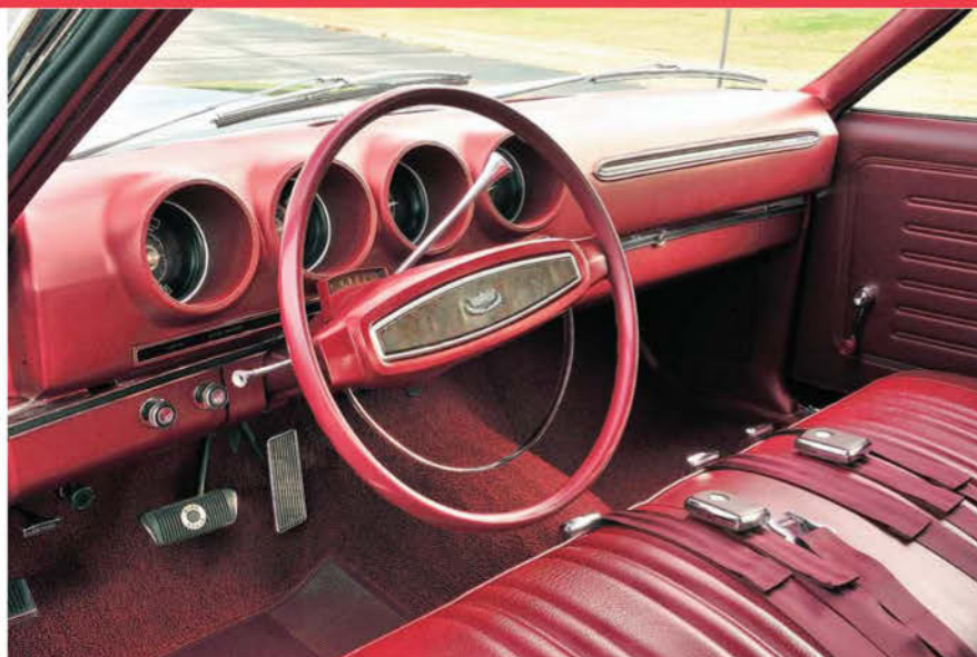
LEFT TOP: Four pods held the Torino's vital gauges. Note this Torino GT has a column-mounted gear shift handle. Ford was sure to note the energy-absorbing steering column and steering wheel for safety.
