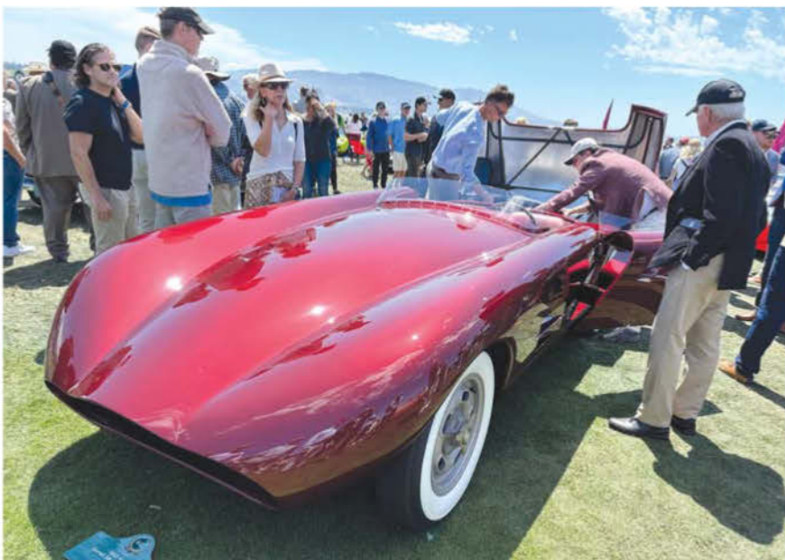
The alloy body of the 1953 Kurtis Sorrell SR-100 at Pebble Beach opens like an aluminum clamshell. Powered by a six-carburetor GMC I-6, this sleek roadster resembled a streamlined Bonneville racer with a windscreen. Haibrand wheels accentuate the car's racing theme.
