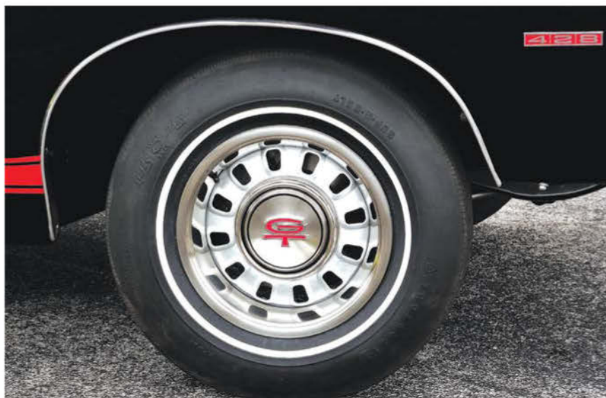
The GT came standard with wide-oval tires; the GT’s standard styled steel wheels were painted a reflective silver paint. Note the “428” fender badge happens to match the GT rocker stripe.
