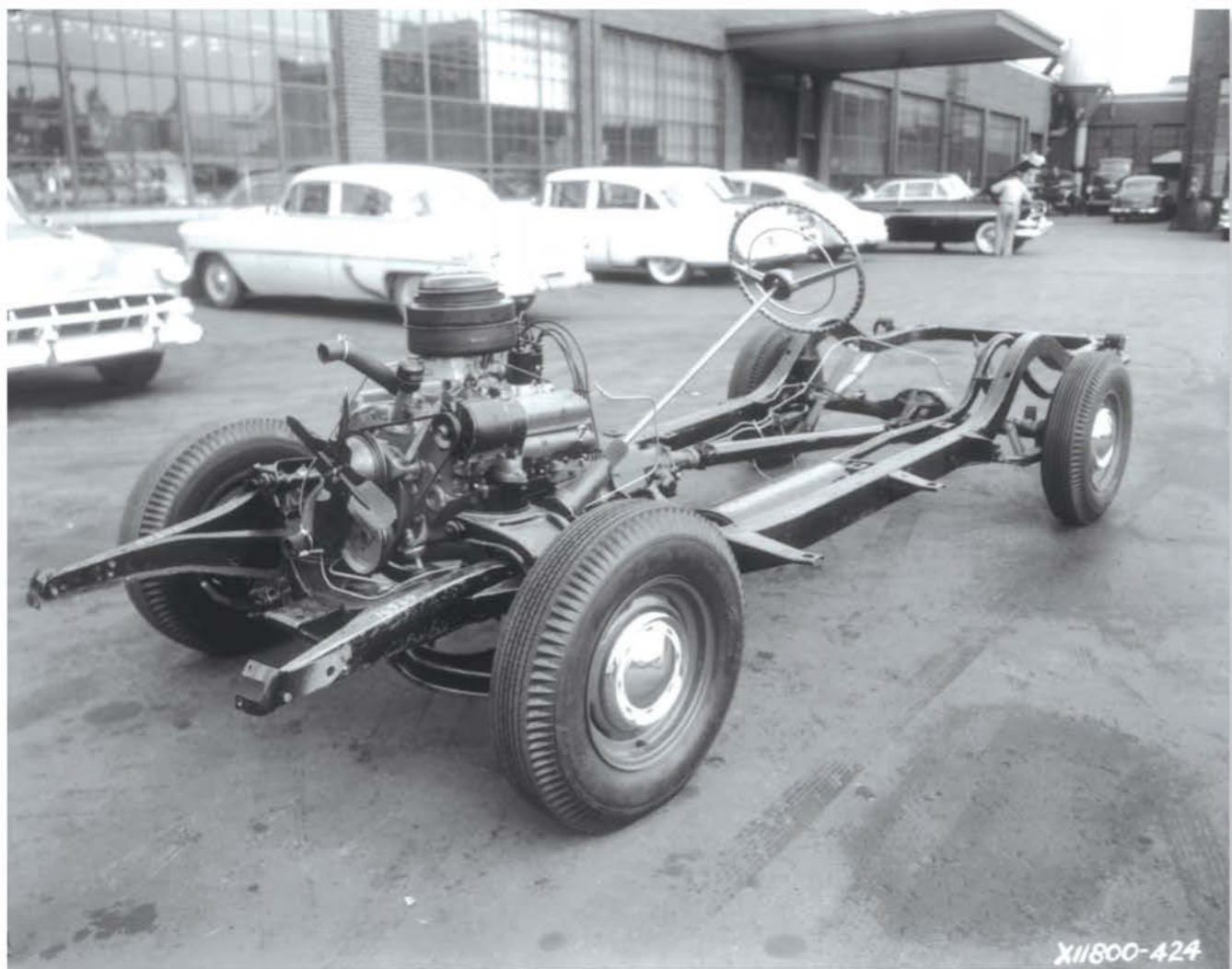
Shown is a prototype 1955 chassis with the complete drivetrain. The front-upper driver's side frame rail has either "16860" or "16960" stenciled in place. Chevy's new chassis design, which marketing described as "Quadra-Poise Ride," contributed to a lower center of gravity, improved weight distribution, and a wider tread, all of which combined "to give a safer, road-hugging ride."
