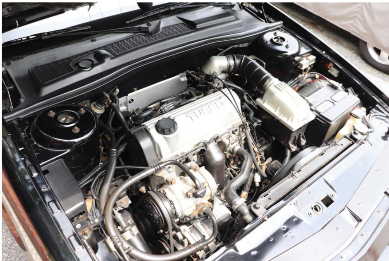
The turbocharged 2.2-liter four-cylinder has remained reliable for its owner over the last three and a half decades.
