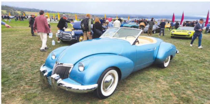
The 1948 Kurtis Omohundro Comet was built by racecar builder Frank Kurtis on a Mercury chassis with a Cadillac flathead V-8. Lost for more than 50 years, this car and a sister roadster were found by the Undiscovered Classics team and carefully restored.
